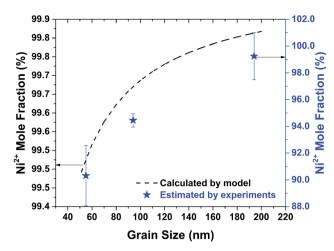
Fig. 6 Mole fractions of Ni<sup>2+</sup> ions estimated from experiments and calculated from thermodynamic model as function of grain size.
