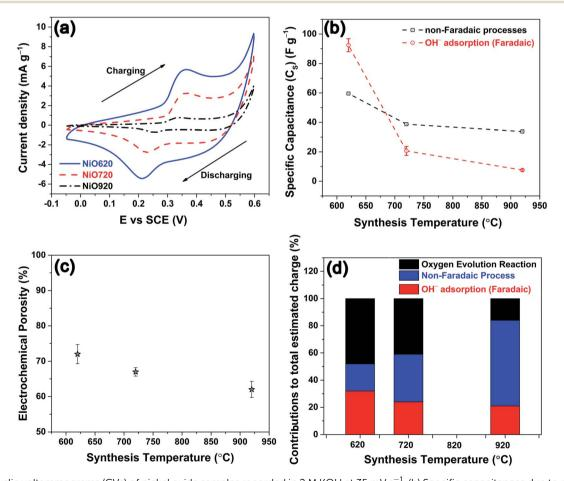
Fig. 4 (a) Cyclic voltammograms (CVs) of nickel oxide samples recorded in 2 M KOH at 35 mV s $^{-1}$ . (b) Specific capacitances due to non-faradaic processes and OH $^-$  adsorption estimated from CVs as function of synthesis temperature. (c) Electrochemical porosity as function of synthesis temperature. (d) Contributions of non-faradaic processes, OH $^-$  adsorption and oxygen evolution reaction to the total estimated charge from CVs.
