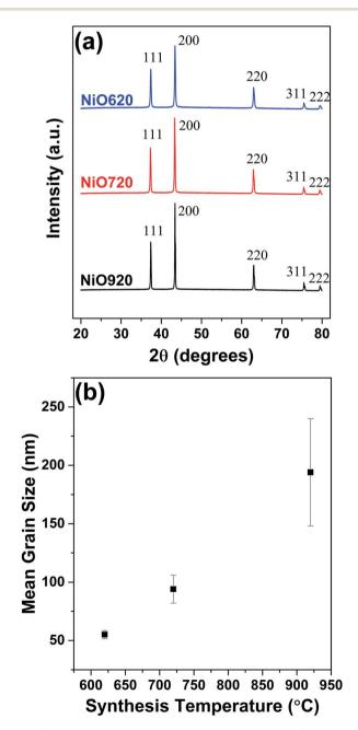
Fig. 1 (a) Powder XRD patterns of nickel oxide powders. (b) Variation of estimated average grain size with synthesis temperature.
