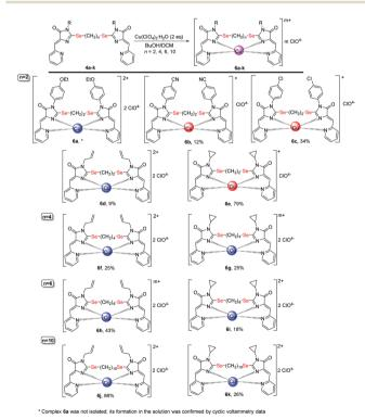
Scheme 7 Coordination compounds 6a-k formed in the reactions of ligands 4 with  $Cu(ClO_4)_2 \cdot 6H_2O$ . The red circles represent  $Cu^{1+}$ , the blue circles represent  $Cu^{2+}$ . The structures of the main reaction products are given, see also Table 1S† and discussion in the text.
