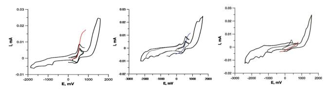
Fig. 5 Cyclic voltammograms of complexes containing  $Cu^{1+}Cu^{1+}$  (compound 5c, left),  $Cu^{1+}Cu^{2+}$  (compound 5a, center) and  $Cu^{2+}Cu^{2+}$  (compound 5i, right). GC electrode, DMF,  $5 \times 10^{-4}$  M, 0.1 M  $Bu_4NClO_4$ . Black curves – CVA, colored curves – RDE.
