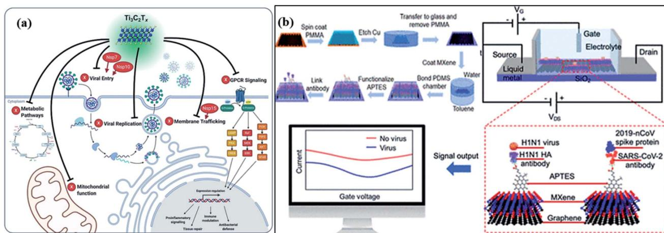
Fig. 8 (a) The mechanism of MXene-dependent viral inhibition of  $\text{Ti}_3\text{C}_2\text{T}_x$  to explore viral inhibition activity at the cell surface, and (b) an illustration of antibody-antigen sensing in a FET circuit and change in the drain-source current is achieved by MXene-graphene VSTM deposition. Photograph: courtesy of "Yanxiao Li". Copyright 2020 and the image is of the free domain.
