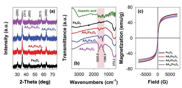
Fig. 1 (a) XRD pattern, (b) FTIR spectra, and (c) magnetization curves of unmodified  $Fe_3O_4$  and the corresponding aspartic-modified  $Fe_3O_4$  nanoparticles.
