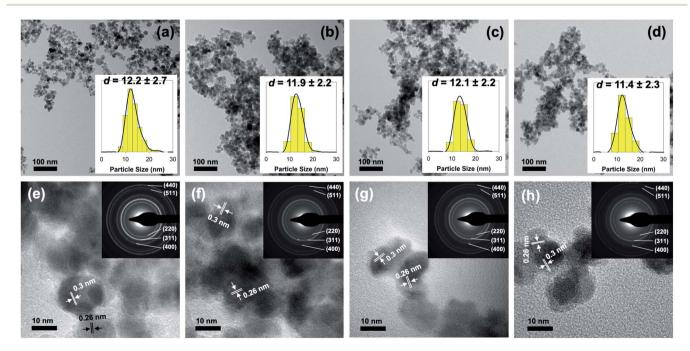
Fig. 2 (a-d) TEM (inset: particle size distributions) and (e-h) HR-TEM images (inset: SAED patterns) of unmodified  $Fe_3O_4$  and the corresponding  $AA_2/Fe_3O_4$ ,  $AA_8/Fe_3O_4$ ,  $AA_{32}/Fe_3O_4$
