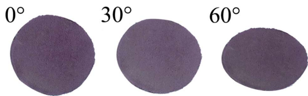
Fig. 12 Optical image of the magenta colored films on CF at different view angles.
