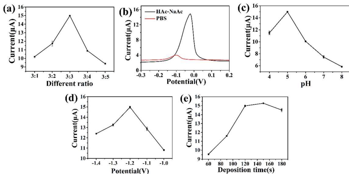
Fig. 5 (a) Peak current comparison of 2.0  $\mu\text{M}$  Cu(II) for the UiO-66-NH<sub>2</sub>/ZnO composite modified electrode with different concentration ratios (U : Z = 3 : 1–3 : 5, U : Z stands for UiO-66-NH<sub>2</sub> : ZnO) in 0.1 M HAC-NaAc solution (pH = 5.0). Influence of various experimental parameters on the DPSV response of UiO-66-NH<sub>2</sub>/ZnO/GCE toward Cu(II) (2  $\mu\text{M}$ ): (b) supporting electrolytes; (c) pH; (d) deposition potential; and (e) deposition time.
