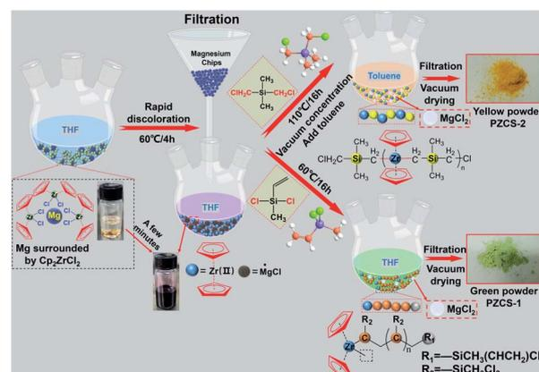
Fig. 1 Synthesis process of PZCS-1 and PZCS-2 precursors.
