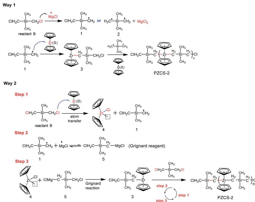
Fig. 3 Possible synthesis pathway of PZCS-2 polymer precursor.
