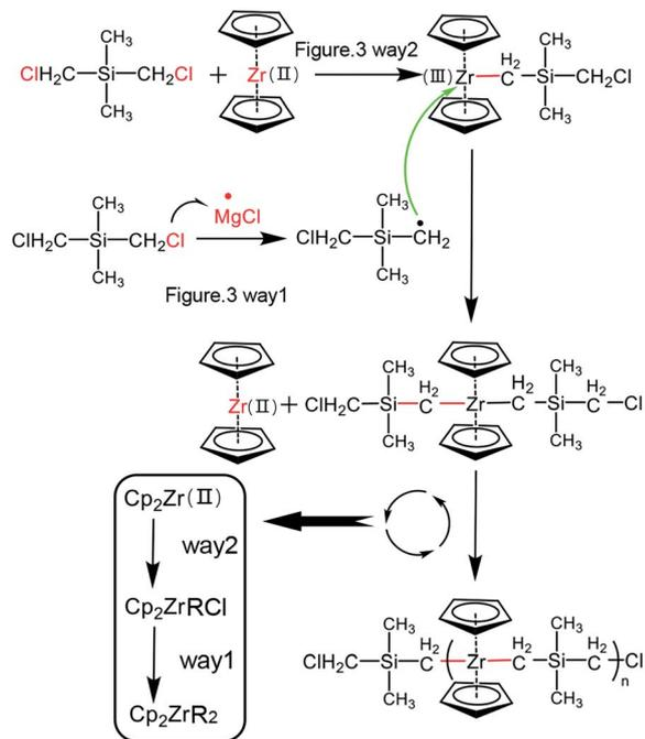
Fig. 5 The synthesis pathway of the PZCS-2 precursor.
