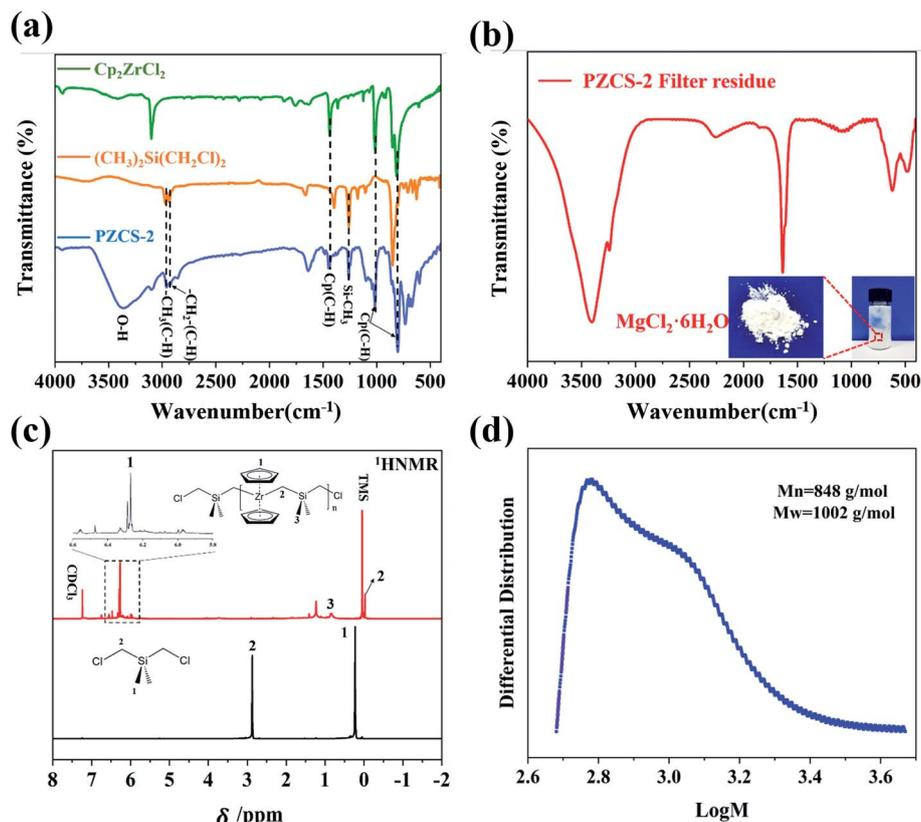
Fig. 2 (a) FTIR spectra of PZCS-2 precursor,  $\text{Cp}_2\text{ZrCl}_2$  and  $(\text{CH}_3)_2\text{Si}(\text{CH}_2\text{Cl})_2$ ; (b) FTIR spectra of PZCS-2 filter residue; (c)  $^1\text{H-NMR}$  spectra of PZCS-2 and  $(\text{CH}_3)_2\text{Si}(\text{CH}_2\text{Cl})_2$  and (d) GPC spectra of PZCS-2 precursor.
