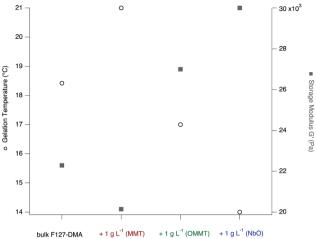
Fig. 7 Evolution of the gelation temperature and the storage modulus of bulk F127-DMA hydrogel and the hydrogel based nanocomposites prepared with MMT, OMMT and NbO at a concentration of 1 g  $\rm L^{-1}$ .
