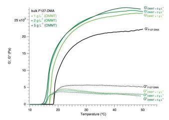
Fig. 4 Changes in both the storage (G', solid line) and loss (G'', dashed line) moduli as a function of temperature for Pluronic F127–H<sub>2</sub>O at a concentration of 25 wt% with PEO chains functionalized by dimethacrylate (DMA) at rate of 88% (black) and reinforced by or including dispersions of an organoclay (OMMT) at concentrations of 1 g L<sup>-1</sup> (light green), 2 g L<sup>-1</sup> (green) and 5 g L<sup>-1</sup> (dark green).
