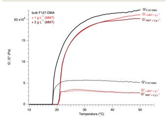
Fig. 3 Changes in both the storage (G', solid line) and loss (G'', dashed line) moduli as a function of temperature for Pluronic F127–H<sub>2</sub>O at a concentration of 25 wt% with PEO chains functionalized by dimethacrylate (DMA) at a rate of 88% (black) and reinforced by or including dispersions of MMT at concentrations of 1 g L<sup>-1</sup> (red) and 2 g L<sup>-1</sup> (dark red).
