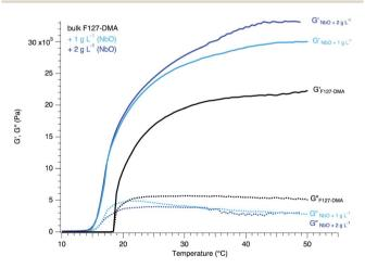
Fig. 5 Changes in both the storage (G', solid line) and loss (G'', dashed line) moduli as a function of temperature for Pluronic F127–H<sub>2</sub>O at a concentration of 25 wt% with PEO chains functionalized by dimethyl acrylate (DMA) at a rate of 88% (black) and reinforced by or including a dispersion of TBA-NbO at concentrations of 1 g L<sup>-1</sup> (light blue) and 2 g L<sup>-1</sup> (dark blue).
