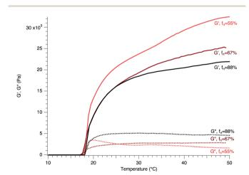
Fig. 2 Changes in both the storage (G', solid line) and loss (G'', dashed line) moduli as a function of temperature for Pluronic F127–H<sub>2</sub>O at a concentration of 25 wt% with PEO chains functionalized by dimethacrylate (DMA) at different rates of 55, 67 and 88% highlighted in red, brown and black colors.
