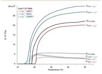
Fig. 6 Changes in both the storage (G', solid line) and loss (G'', dashed line) moduli as a function of temperature for Pluronic F127–H<sub>2</sub>O at a concentration of 25 wt% with PEO chains functionalized by dimethyl acrylate (DMA) at a rate of 88% (black) and reinforced by dispersions of MMT (dark red), NbO (blue) and OMMT (green) at a concentration of 1 g L<sup>-1</sup>.
