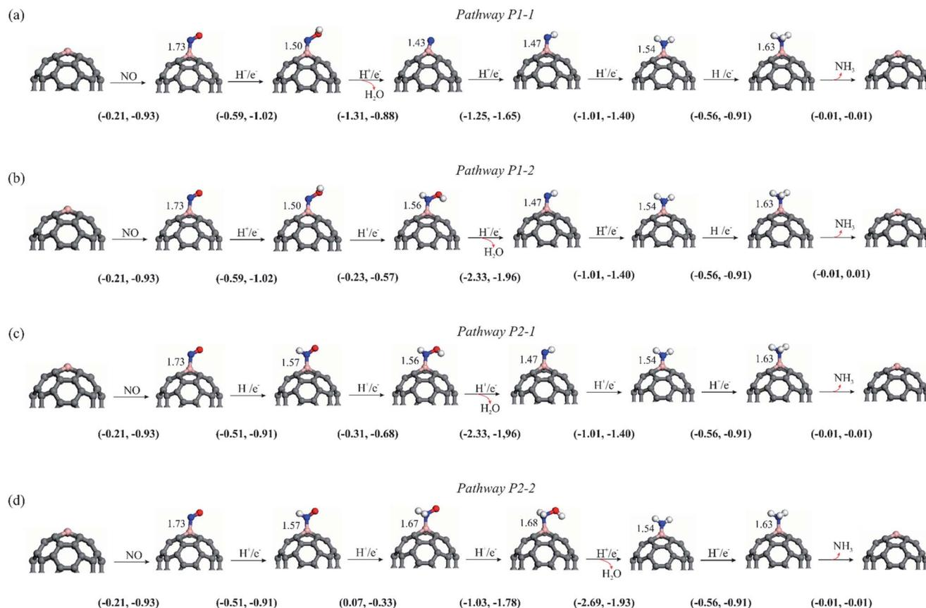
Fig. 5 Optimized structure of various intermediates for NOER to  $\text{NH}_3$  along the (a) P1-1, (b) P1-2, (c) P2-1 and (d) P2-2 pathways over  $\text{C}_{59}\text{B}$ . All B–N bond distances are in Å. The first number in the parentheses is the  $\Delta G$ , while the second is the  $\Delta E$ .
