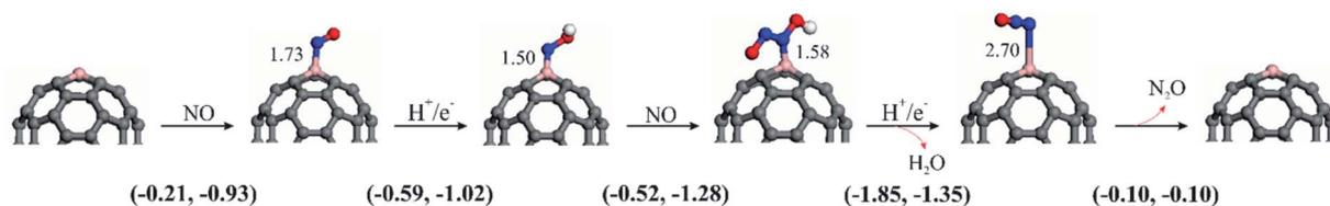
Fig. 6 Optimized structures of NOER species over  $\text{C}_{59}\text{B}$  at high NO coverage. All B–N bond distances are in Å. All B–N bond distances are in Å. The first number in the parentheses is the  $\Delta G$ , while the second is the  $\Delta E$ .
