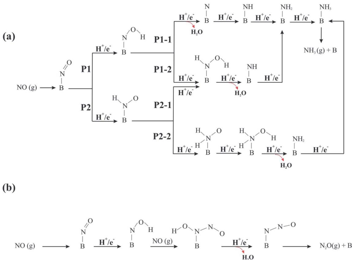
Fig. 4 Schematic representation of possible reaction pathways for NOER process over C<sub>59</sub>B at (a) low and (b) high NO coverage.
