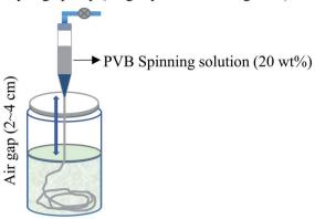
TTIP coagulation bath solution (5 wt%~50 wt%)
