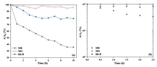
Fig. 17 (a) The capacity of adsorbed MB, MO, and Rh-B dyes in the dark, and (b) dye decomposition ability in visible light irradiation for 20 wt% PVB-amTiO<sub>2</sub>F, reaction conditions: fiber 0.2 g, 10 mL (10 mg L<sup>-1</sup>) dyes, pH  $\sim$  8.0, at 18 °C.
