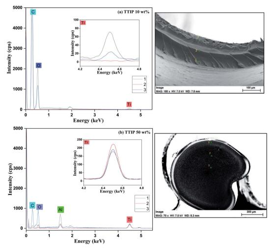
Fig. 8 Point analysis of EDS for the PVB-amTiO $_2$ F samples. 3 analysis points were indicated by green cross in the right-side pictures; point 1 indicates the surface, point 2 indicates the intermediates of the other two and point 3 indicates the center position of the fiber cross-section. Al might appear from the sample holder. The magnified plot (inset) illustrates more Ti distribution at center points for both fibers.
