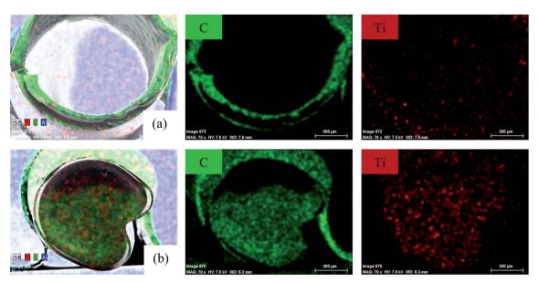
Fig. 7 EDX elemental mapping of PVB-amTiO $_2$ F cross-sections prepared with (a) 10 wt% TTIP bath concentrations, and (b) 50 wt% TTIP bath concentrations.
