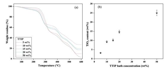
Fig. 4 (a) Typical TG profiles, and (b) residual TiO<sub>2</sub> weight of the PVB-amTiO<sub>2</sub>F samples at 600 °C as a function of TTIP bath concentration.
