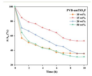
Fig. 13 The adsorption dynamics of MB in different reaction systems, when the samples were immersed into the MB solutions in the dark. Reaction conditions: Fiber: 0.2 g, 10 mL (10 mg  $L^{-1}$ ) MB, pH  $\sim$  8.0, at 18 °C.
