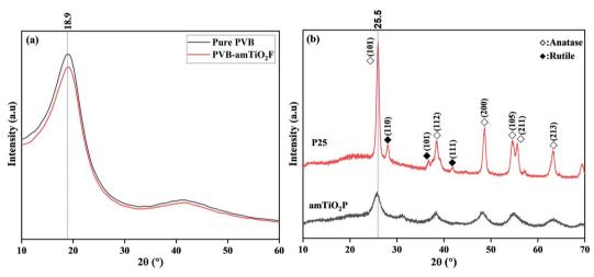
Fig. 6 XRD patterns of (a) pure PVB and PVB-amTiO<sub>2</sub>F; and (b) synthesized amTiO<sub>2</sub>P and P25
