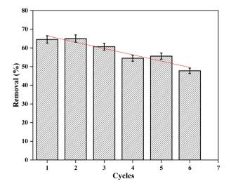
Fig. 19 Reusability of PVB-amTiO<sub>2</sub>F in MB adsorption.
