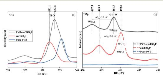
Fig. 10 XP spectra of pure PVB, amTiO<sub>2</sub>P, and PVB-amTiO<sub>2</sub>F; (a) O1s spectra, and (b) Ti2p.
