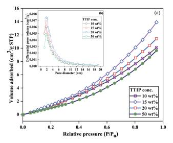
Fig. 11 (a)  $N_2$  adsorption isotherms ( $-196\,^{\circ}$ C), and (b) the corresponding BJH pore size distribution plots of PVB-amTiO<sub>2</sub>F with different TTIP bath concentrations.
