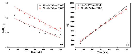
Fig. 14 The adsorption kinetic plots of MB on PVB-amTiO<sub>2</sub>F fitted with (a) pseudo-first-order, and (b) pseudo-second-order models.
