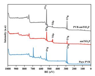
Fig. 9 Wide-scan XP spectra of pure PVB,  $amTiO_2P$ , and PVB- $amTiO_2F$ .
