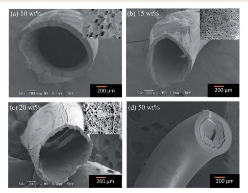
Fig. 2 SEM images of the PVB-amTiO<sub>2</sub>F prepared at TTIP bath concentrations of (a) 10 wt%, (b) 15 wt%, (c) 20 wt%, and (d) 50 wt%.
