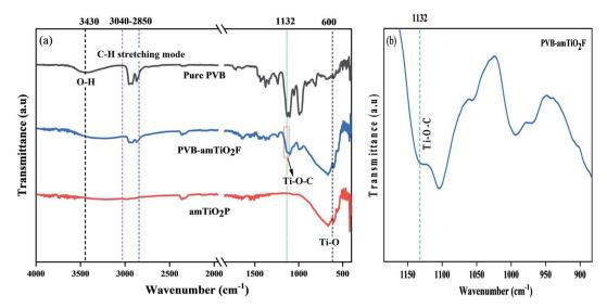
Fig. 5 ATR-FTIR spectra of (a) pure PVB, amTiO<sub>2</sub>P, and PVB-amTiO<sub>2</sub>F; and (b) considered coordinate bonding position in PVB-amTiO<sub>2</sub>F.
