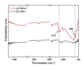
Fig. 18 ATR-FTIR spectra of PVB-amTiO $_2$ F (a) before, and (b) after MB adsorption.
