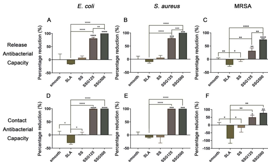
Fig. 8 The percentage reduction of *E. coli*, *S. aureus*, and MRSA in release and contact antibacterial experiment of different samples. (\* $p < 0.05$ , \*\* $p < 0.01$ , \*\*\* $p < 0.005$ , \*\*\*\* $p < 0.0001$ ).
