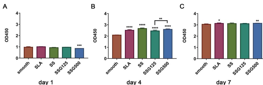
Fig. 6 Proliferation of MC3T3-E1 cells culturing with the samples of Smooth, SLA, SS, SSG125, and SSG500 groups. (\* $p < 0.05$ , \*\* $p < 0.01$ , \*\*\* $p < 0.005$ , \*\*\*\* $p < 0.0001$ ).
