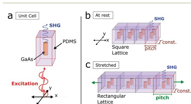
**Fig. 1** (a) Schematic of the periodic structure that is implemented in the finite element model. It consists of a unit cell with PDMS and a NW of specific length and diameter in the centre. (b) NW array at rest configuration and (c) under uniaxial stretching, for which the size of the unit cell varies only in one direction. A plane wave with linear polarization ( $x$ - or  $y$ -polarization) excites the GaAs NWs, generating SH.
