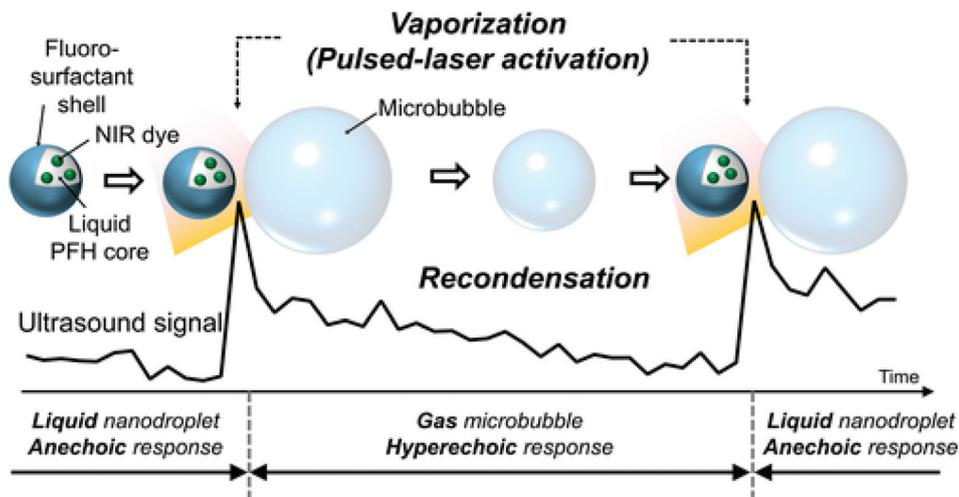
**Fig. 8** Vaporisation and recondensation of laser-activated nanodroplets. When activated, nanodroplets immediately produce strong ultrasound signals<sup>107</sup> (this figure has been reproduced from ref. 107 with permission from John Wiley and Sons, copyright 2017).
