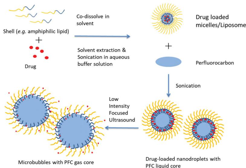
Fig. 5 Schematic representation of the preparation of PCND and their phase change with focused ultrasound.
