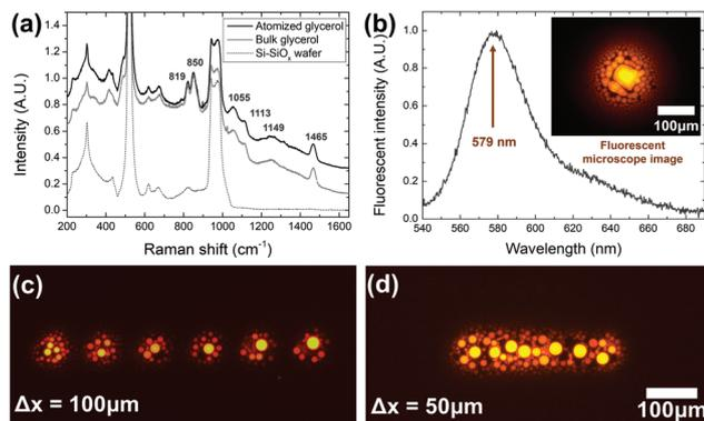
**Fig. 4** (a) Raman spectra of the Si-SiO<sub>x</sub> wafer, atomized, and bulk glycerol from the optical atomizer. (b) The fluorescent spectrum of the atomized glycerol-rhodamine B solution with 3 g L<sup>-1</sup> concentration. The inset shows the fluorescent microscope image. Fluorescent microscope image of the six shots of the atomized glycerol-rhodamine B solution with consistent interval  $\Delta x$  of (c) 100  $\mu\text{m}$  and (d) 50  $\mu\text{m}$ .
