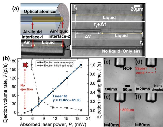
**Fig. 2** (a) Air–liquid interfaces for measuring optofluidic properties of the optical atomizer. The enlarged bright-field microscope image shows the liquid filled inside the capillary of HOF. (b) The ejection volume rate and ejection initiating time as a function of the laser power absorbed by the SWCNT thin film. (c–f) The nano-droplets from the atomizer were recorded using a high-speed camera. The absorbed laser power is 19 mW.
