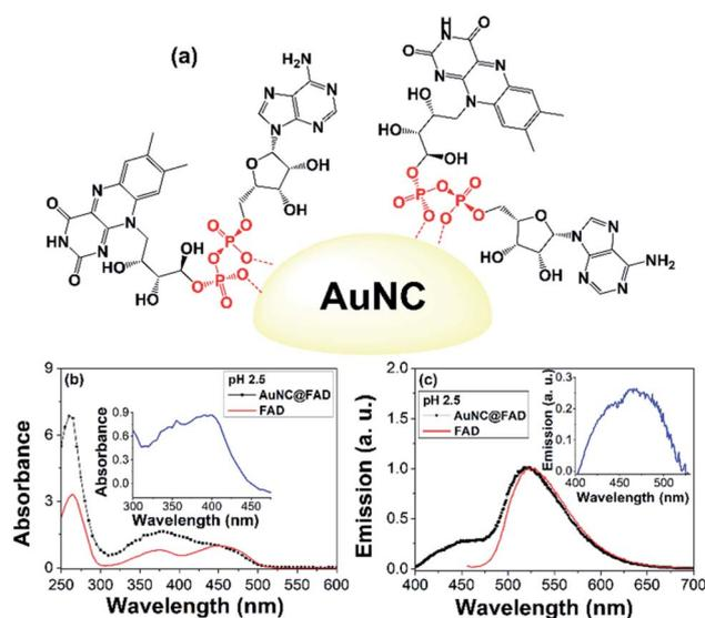
Fig. 1 (a) Pictorial representation of the binding of FAD in AuNC@FAD. (b) Absorption and (c) emission spectra ( $\lambda_{exc} = 390$  nm) of AuNC@FAD in water at pH 2.5 (in black) compared to those of FAD in water (in red); insets: difference (b) absorption and (c) emission spectra.
