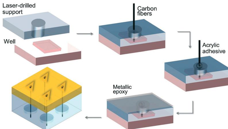
Fig. 3 Schematic illustration of the hybrid microneedle developed by Miller *et al.*<sup>61</sup>
