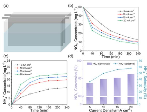
**Fig. 5** (a) Schematic of the pilot-scale electrochemical reactor. The concentrate-time curves of (a) nitrate and (b) ammonium over Cu-Fe<sub>2</sub>O<sub>3</sub>-60. (c) The nitrate conversion rate and ammonium selectivity of Cu-Fe<sub>2</sub>O<sub>3</sub>-60 under different current densities.
