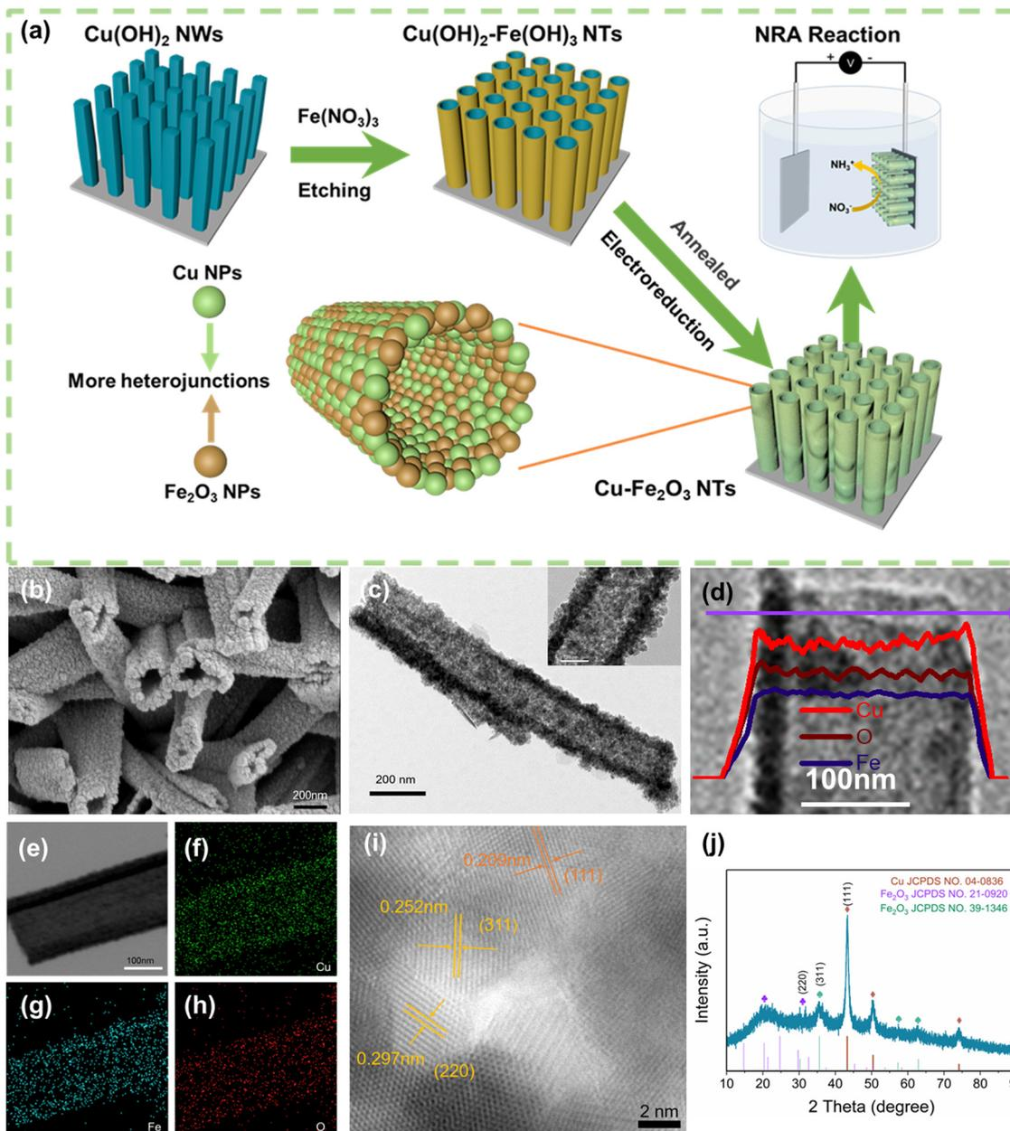
Fig. 1 (a) Schematic of defective Cu-Fe<sub>2</sub>O<sub>3</sub> synthesis. (b) The SEM image (c) TEM image, (d) elemental concentration profile images, (e–h) elemental mapping images, (i) HR-TEM image, (j) XRD pattern of Cu-Fe<sub>2</sub>O<sub>3</sub>-60.
