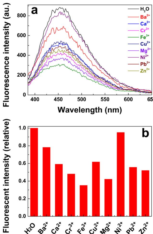
Fig. 9 Fluorescence response of the poly(AM-co-AA)/GQD nanocomposite hydrogels (1 wt% GQDs) to different ions dissolved in deionized water: (a) fluorescence spectra and (b) corresponding relative fluorescence intensity.
