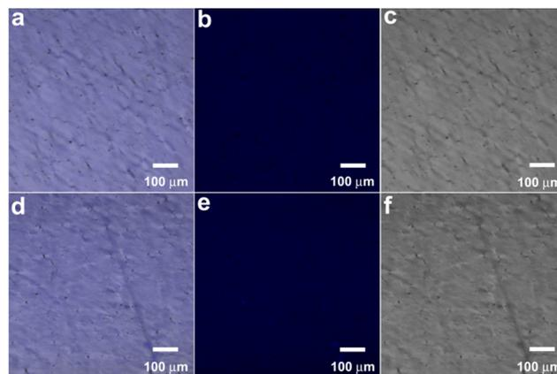
Fig. 10 Fluorescence images of poly(AM-co-AA)/GQD nanocomposite hydrogels (1 wt% GQDs) under irradiation at 405 nm ((a–c) without and (d–f) 30 min after FeCl<sub>3</sub> was added). (a and d) The images after superposition of both light field and dark field. (b, e and d, f) Images of the light field and dark field, respectively.
