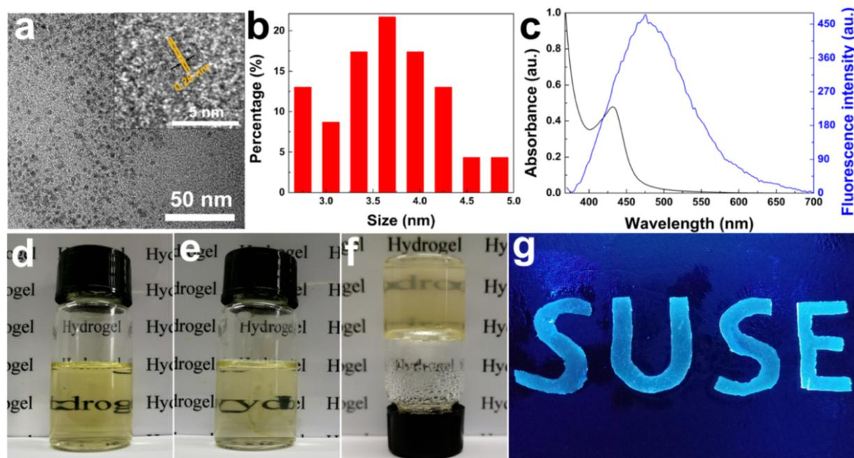
**Fig. 1** (a) TEM image (inset: HRTEM image of GQDs showing lattice spacing), (b) size histogram (counting 100 particles at least), and (c) UV-Vis absorbance and fluorescence emission spectra of synthesised GQDs (1 wt%); preparation of poly(AM-co-AA)/GQD nanocomposite hydrogels ((d) optical images of an aqueous GQD dispersion, (e) GQD dispersion mixed with AM and AA, (f) nanocomposite hydrogels). (g) The obtained hydrogels exhibited obvious blue fluorescence under 365 nm UV light.
