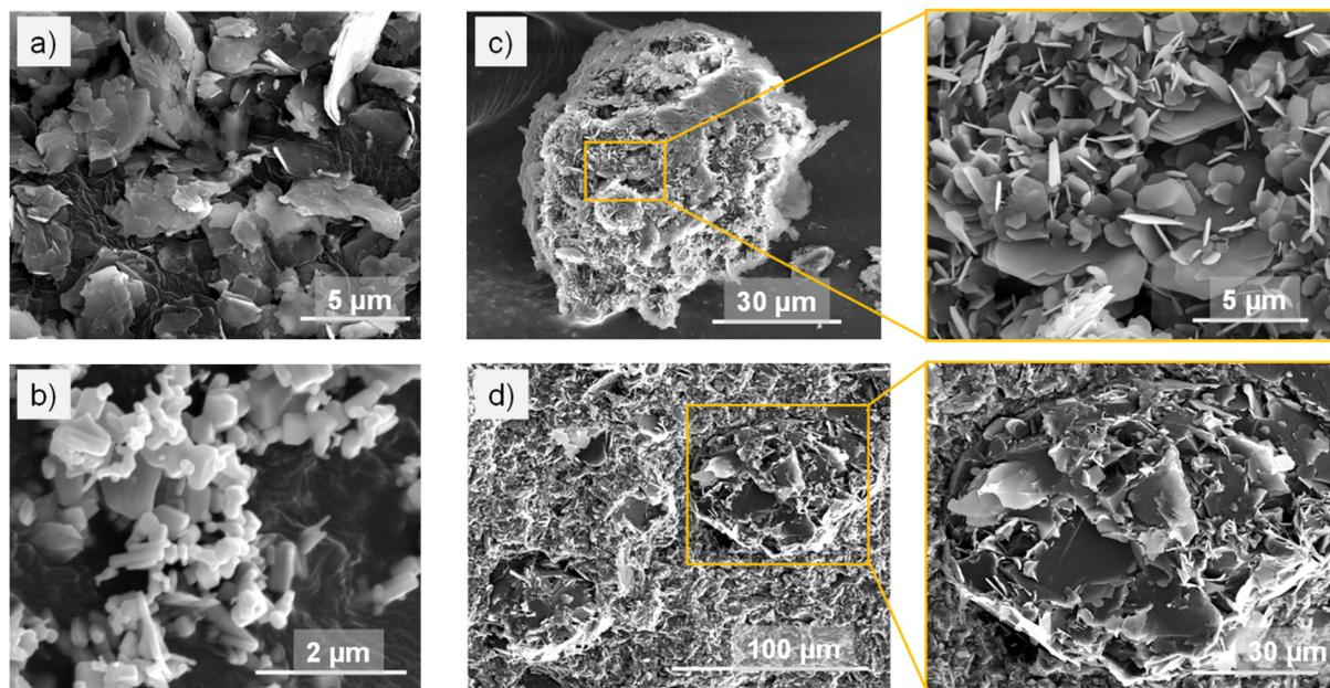
**Fig. 1** SEM images of as-received functional fillers and an epoxy composite. (a) Talc platelets; (b) ZnO particles; (c) BN cluster particle PTX 60 with magnification showing edge-connecting BN platelets; (d) cross-section of an epoxy composite formulation, magnification – a BN cluster in the composite.
