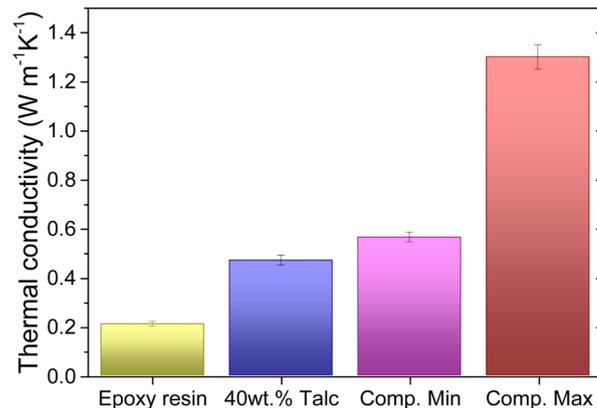
Fig. 3 Enhancement in thermal conductivity of the epoxy composite.
