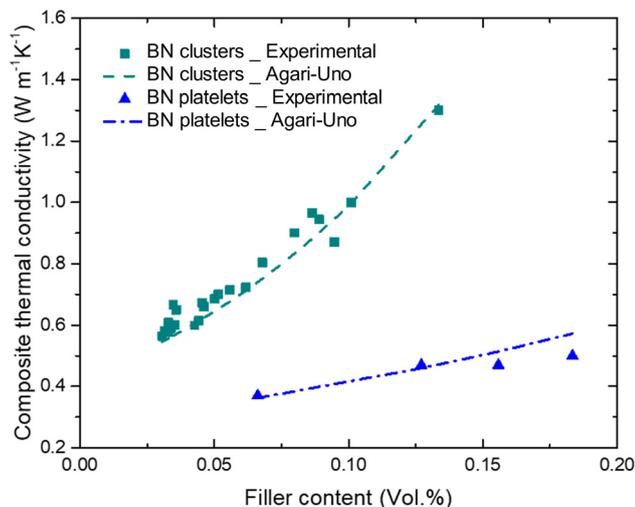
Fig. 6 Thermal conductivity of epoxy/BN clusters and epoxy/BN platelets composite and fits for the Agari-Uno model.
