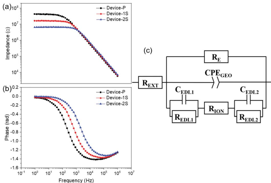
Fig. 2 EIS curves of  $\text{Ru}(\text{bpy})_3(\text{PF}_6)_2$  memristor devices with different concentrations of  $\text{LiClO}_4$ . (a) Impedance versus frequency data and (b) phase versus frequency data for Device-P (black squares), Device-1S (red circles), and Device-2S (blue triangles). (c) An equivalent circuit employed for EIS fitting of the OMIEC memristor devices.
