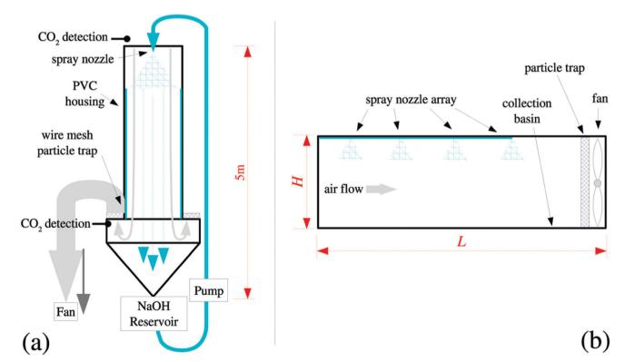
Fig. 23 Representation of off-the-shelf spray contactor for DAC. Taken from ref. 356. Reprinted (adapted) with permission from Stolaroff et al., Carbon dioxide capture from atmospheric air using sodium hydroxide spray, Environ. Sci. Technol., 42, 2728–2735. Copyright 2008 American Chemical Society
