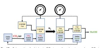
Fig. 19 Schematic of a biphasic CO<sub>2</sub> to methanol system, where CO<sub>2</sub> is captured and converted from the air and the amine and catalyst are recyclable. Taken from ref. 337. Reprinted (adapted) from Kar et al., Integrative CO<sub>2</sub> capture and hydrogenation to methanol with reusable catalyst and amine: Toward a carbon neutral methanol economy, J. Am. Chem. Soc., 140, 1580-1583. Copyright 2018 American Chemical Society.
