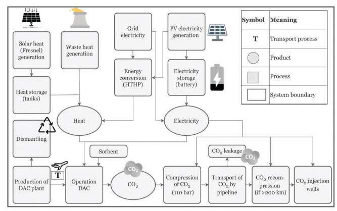
Fig. 27 Superstructure of the process boundaries for life-cycle emissions of DAC. Taken from ref. 171. Reprinted (adapted) with permission from Terlouw et al., Life cycle assessment of direct air carbon capture and storage with low-carbon energy sources, Environ. Sci. Technol., 55, 11397-11411. Copyright 2021 American Chemical Society
