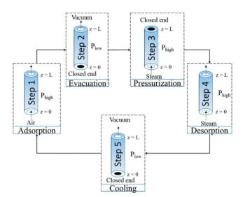
Fig. 25 Temperature vacuum swing adsorption for DAC. Taken from ref. 284. Reprinted (adapted) with permission from Sinha et al., Systems design and economic analysis of direct air capture of CO<sub>2</sub> through temperature vacuum swing adsorption using MIL-101(Cr)-PEI-800 and mmen-Mg<sub>2</sub>(dobpdc) MOF adsorbents, Ind. Eng. Chem. Res., 56, 750-764. Copyright 2017 American Chemical Society.
