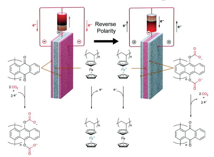
Fig. 17 Electro-swing adsorption of CO<sub>2</sub>. Following the application of a reducing potential, carboxylation of quinone captures CO<sub>2</sub>. CO<sub>2</sub> is released when the polarity is reversed. The inner polyvinylferrocene-containing electrode acts as an electron source and sink. Reproduced from ref. 318 with permission from the Royal Society of Chemistry
