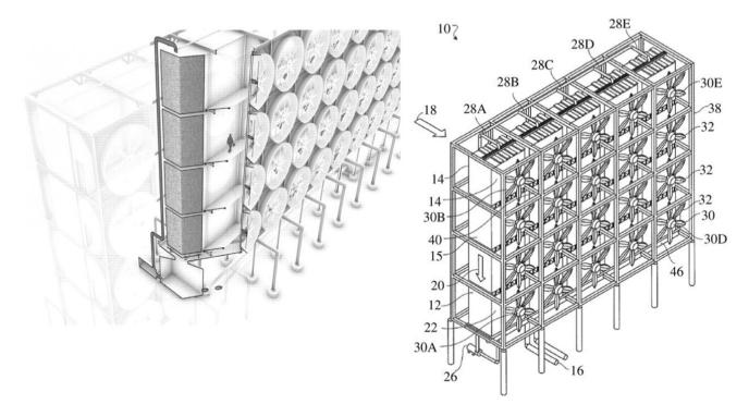
Fig. 12 The Carbon Engineering contactor design featuring forced-draft fans and structure packing with cross-flow gas and a liquid feed. Taken from ref. 281 Republished with permission of The Royal Society (UK), from An air-liquid contactor for large-scale capture of CO<sub>2</sub> from air, Holmes and Keith, 370, 1974, 2012; permission conveyed through Copyright Clearance Centre, Inc.
