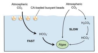
Fig. 18 DAC by microalgae, catalysed by carbon anhydrase. Buoyant beads containing carbonic anhydrase float at the gas-liquid interface, acting as a catalyst for the CO<sub>2</sub> to bicarbonate reaction. Taken from ref. 335. Reprinted (adapted) with permission from Xu et al., Direct air capture of CO<sub>2</sub> by microalgae with buoyant beads encapsulating carbonic anhydrase, ACS Sustainable Chem. Eng., 9, 9698-9706. Copyright 2021 American Chemical Society
