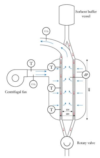
Fig. 14 Moving-bed contactor. Blue arrows indicate gas flow and red arrows indicate solid sorbent flow. Taken from CO2 Capture from air in a radial flow contactor: Batch or continuous operation? ref. 294, licensed under CC BY 4.0
