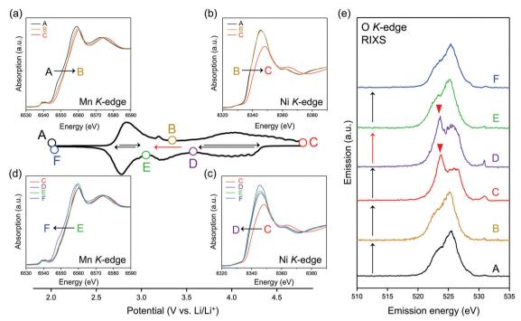
Fig. 2 Redox couples in  $O2-Li_{1.12-y}Ni_{0.17}Mn_{0.71}O_2$ . dQ/dV plot during the second cycle at a charge/discharge rate of C/20. (a–d) Ex situ Mn and Ni K-edge X-ray absorption spectra upon charge and discharge. (e) Ex situ O K-edge resonant inelastic X-ray scattering (RIXS) spectra excited by an incident photon energy of 531 eV.
