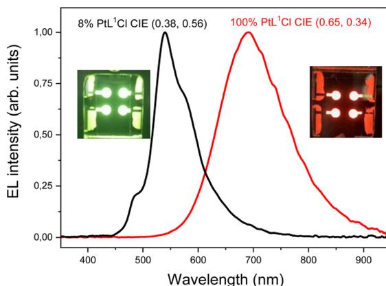
**Fig. 4** (a) Luminance vs. applied voltage and external EL efficiency vs. current density (inset) of the OLEDs. (b) Electroluminescence spectra at 7 V of OLEDs. In the inset there are photos of yellow-green and deep red OLEDs based on  $[\text{PtL}^1\text{Cl}]$ .
