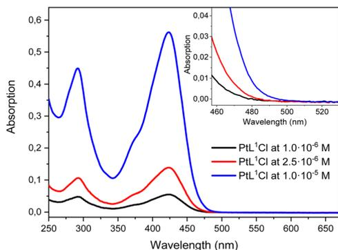
**Fig. 1** Absorption spectra at different concentrations of **[PtL<sup>1</sup>Cl]**, **[PtL<sup>2</sup>Cl]** and **[PtL<sup>3</sup>Cl]** in CH<sub>2</sub>Cl<sub>2</sub> at 298 K. The weak bands at longer wavelengths are shown on an expanded scale for clarity.
