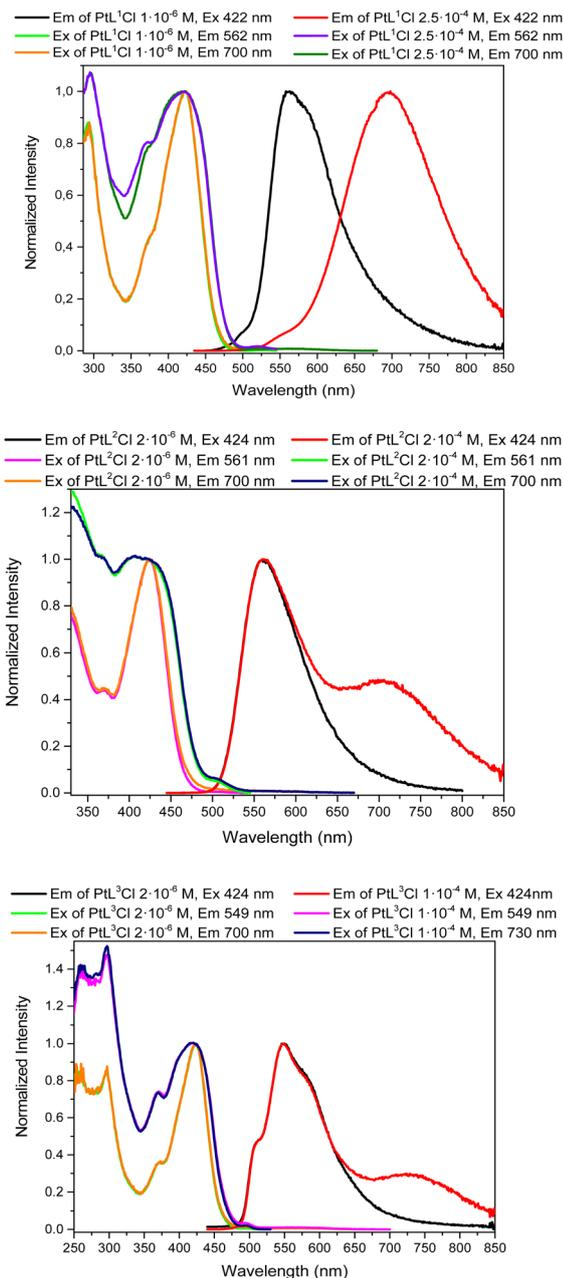
**Fig. 2** Normalized emission and excitation spectra of diluted and concentrated solutions of  $[\text{PtL}^1\text{Cl}]$ ,  $[\text{PtL}^2\text{Cl}]$  and  $[\text{PtL}^3\text{Cl}]$  in  $\text{CH}_2\text{Cl}_2$  at 298 K.
