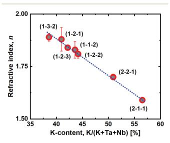
Fig. 8 Refractive index, n, as a function of the film potassium cation content. The blue dashed line is a linear fit of the measured data
