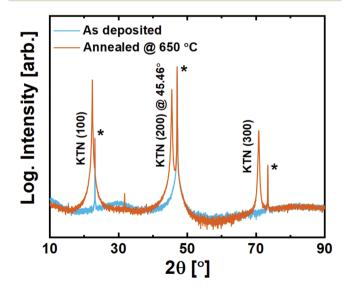
Fig. 9 X-ray diffraction of 200 nm KTa<sub>0.67</sub>Nb<sub>0.35</sub>O<sub>3</sub> thin films deposited on LSAT (100) substrates. Substrate reflections are marked with\*.
