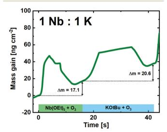
Fig. 6 QCM campaign for a supercycle of 1:1 (Nb:K), showing the mass gain per time for the unique subcycles.
