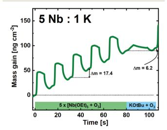
Fig. 5 QCM campaign for a supercycle of 5:1 (Nb:K), showing the mass gain per time for the unique subcycles.
