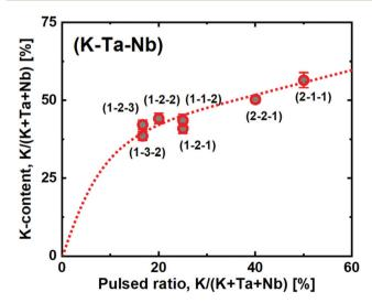
Fig. 7 Potassium content as a function of the pulsed ratio of KO<sup>t</sup>Bu, showing rapid K-incorporation at low ratios before responding linearly. Dashed red line is a guide of eye, error bars are based on reported confidence in XRF measurements.
