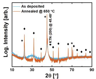
Fig. 10 X-ray diffraction of 200 nm  $KTa_{0.67}Nb_{0.35}O_3$  thin films deposited on MgAl<sub>2</sub>O<sub>4</sub> (100) substrates. Substrate reflections are marked with \*, while perovskite film reflections are marked with  $\spadesuit$ .
