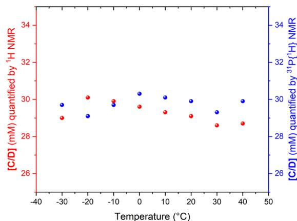
Fig. 3 Concentration of C/D quantified by selective excitation <sup>1</sup>H and <sup>31</sup>P{<sup>1</sup>H} NMR spectroscopy in the mixture containing 40 mM of [RhH(CO)(PPh<sub>3</sub>)<sub>3</sub>], 10 mM of TMB and 10 mM of TPOP in 0.8 mL of non-deuterated toluene under argon.
