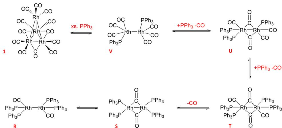
**Scheme 4** Equilibria of  $\text{Rh}^0$  dimer formation from  $[\text{Rh}_4(\text{CO})_{12}]$  with  $\text{PPh}_3$  and  $\text{CO}$  in toluene (covalent  $\text{Rh}-\text{Rh}$  interactions render the  $d^9$  systems diamagnetic and thus NMR active).
