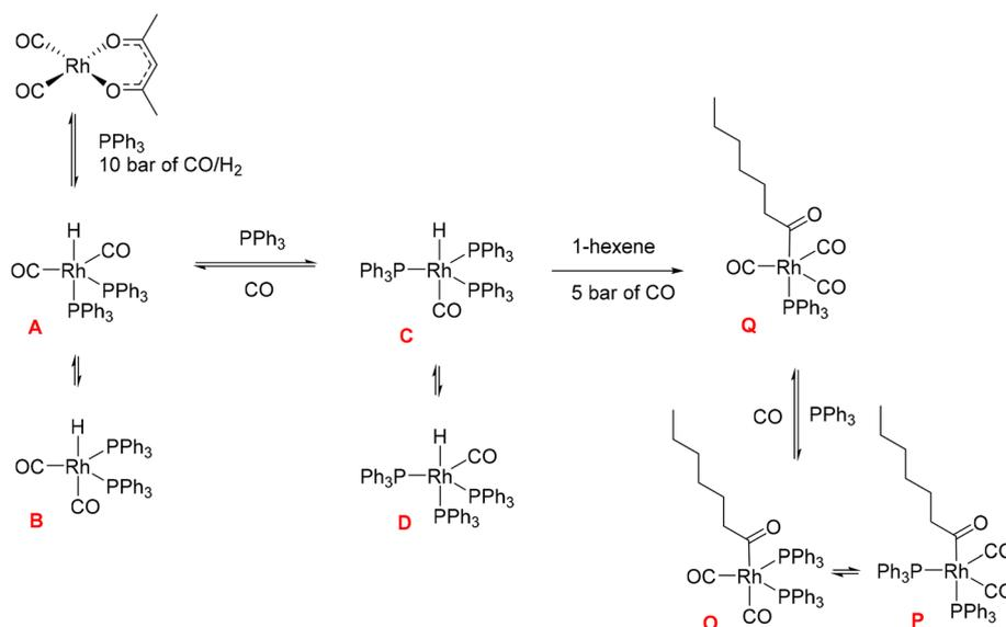
**Scheme 1** Phosphine Rh complexes detected and characterised by FlowNMR spectroscopy when monitoring the hydroformylation of 1-hexene in the presence of Rh(acac)(CO)<sub>2</sub>/PPh<sub>3</sub> at 50 °C in toluene.<sup>28</sup>
