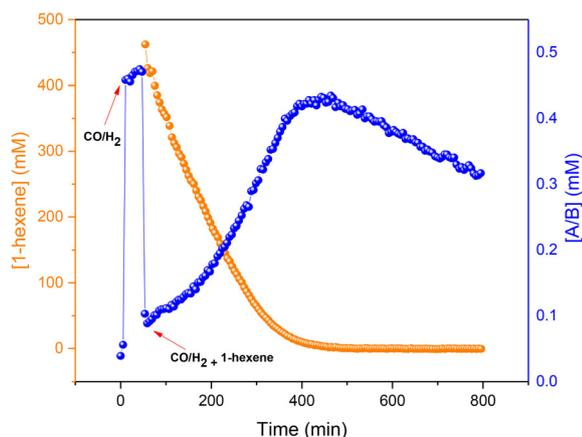
**Fig. 18** Profiles of A/B and substrate during the hydroformylation of 1-hexene under 10 bar of  $\text{CO}/\text{H}_2$  (1:1) at  $50^\circ\text{C}$  starting with  $[\text{C}] = 2.5$  mM in 22.4 mL of non-deuterated toluene as derived from quantitative FlowNMR.
