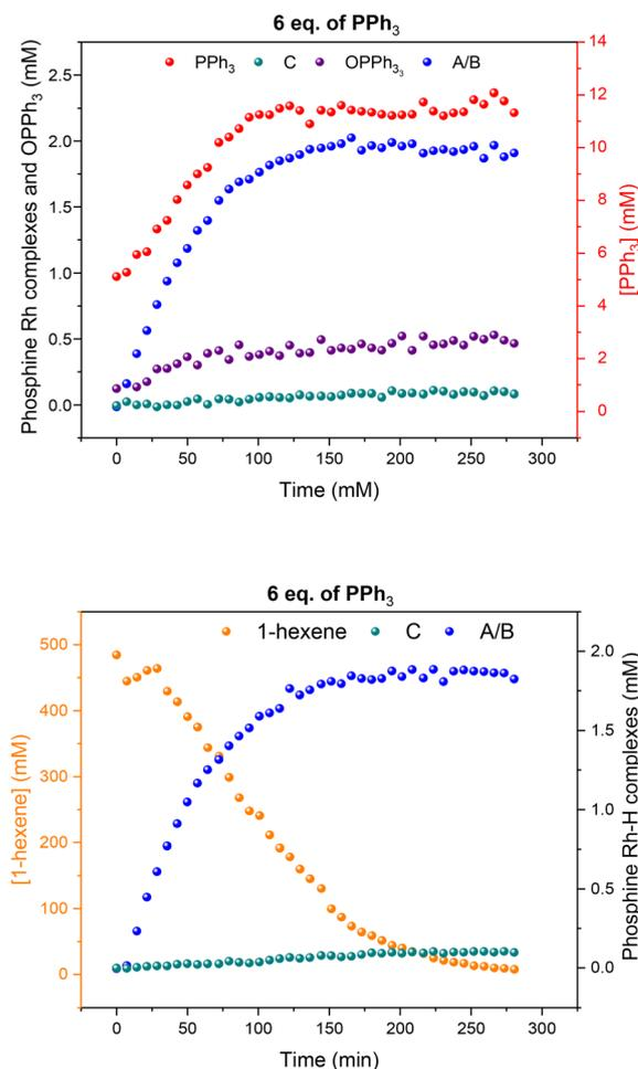
**Fig. 13** Profiles of catalyst species from quantitative  $^{31}\text{P}\{^1\text{H}\}$  FlowNMR (upper) and 1-hexene concentration from quantitative  $^1\text{H}$  FlowNMR (lower) during the hydroformylation of 1-hexene under 10 bar of CO/H<sub>2</sub> (1:3) at 50 °C catalysed by  $[\text{Rh}(\text{acac})(\text{CO})_2] = 2.5$  mM and  $[\text{PPh}_3] = 15$  mM in 22.4 mL of non-deuterated toluene using the temperature gradients shown in Fig. 7.
