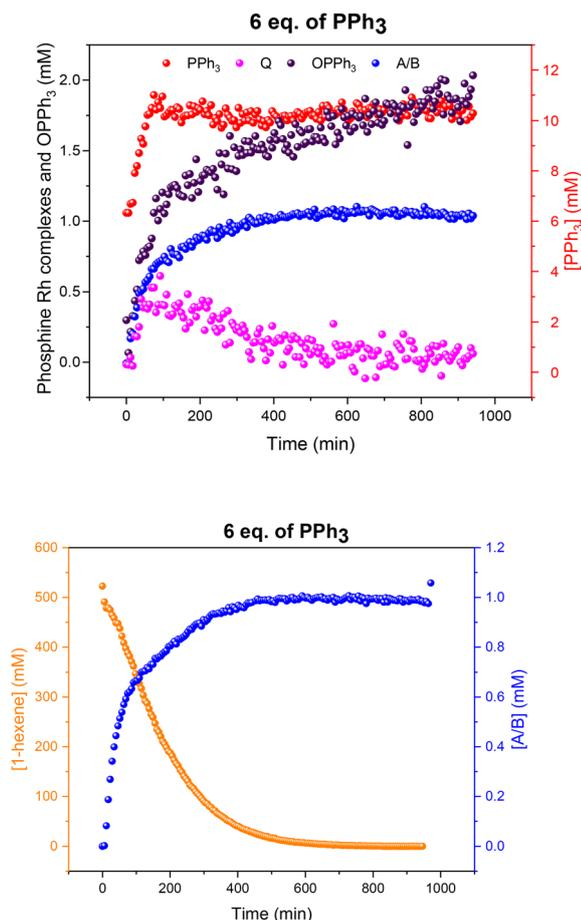
**Fig. 12** Profiles of catalyst species from quantitative  $^{31}\text{P}\{^1\text{H}\}$  FlowNMR (upper) and 1-hexene concentration from quantitative  $^1\text{H}$  FlowNMR (lower) during the hydroformylation of 1-hexene under 10 bar of CO/H<sub>2</sub> (1:1) at 50 °C catalysed by  $[\text{Rh}(\text{acac})(\text{CO})_2] = 2.5$  mM and  $[\text{PPh}_3] = 15$  mM in 22.4 mL of non-deuterated toluene using the temperature gradients shown in Fig. 7.
