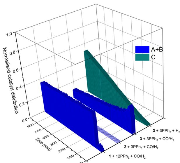
Fig. 17 Activation of different Rh precursors (Fig. 16) at 2.5 mM in toluene with  $\text{PPh}_3$  and  $\text{H}_2$  and/or  $\text{CO}$  at 10 bar and 50 °C as derived from quantitative FlowNMR spectroscopy.
