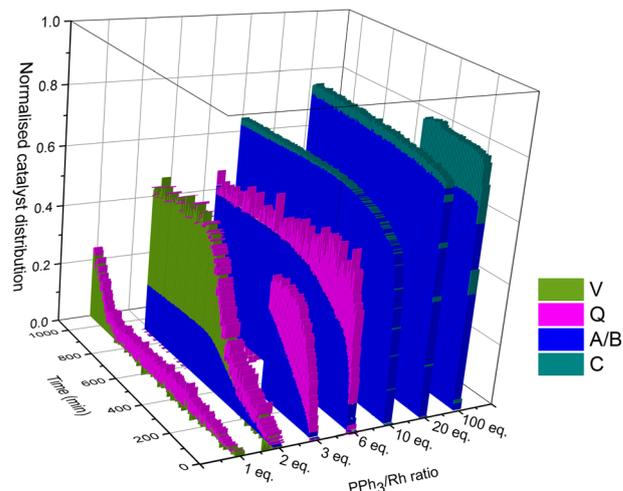
**Fig. 15** Comparison of Rh speciation over time during the hydroformylation of 1-hexene under 10 bar of  $\text{CO}/\text{H}_2$  (1:1) at 50 °C catalysed by  $[\text{Rh}(\text{acac})(\text{CO})_2] = 2.5$  mM with varying amounts of  $\text{PPh}_3$  in toluene as derived from quantitative FlowNMR spectroscopy.
