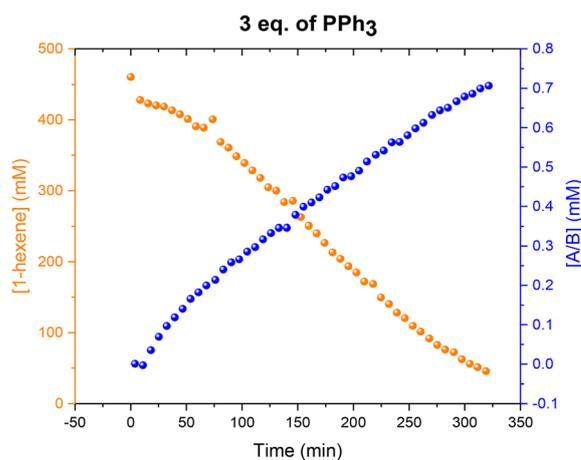
Fig. 11 Profiles of catalyst species from quantitative  $^{31}\text{P}\{^1\text{H}\}$  FlowNMR (upper) and 1-hexene concentration from quantitative  $^1\text{H}$  FlowNMR (lower) during the hydroformylation of 1-hexene under 10 bar of  $\text{CO}/\text{H}_2$  (1:1) at  $50^\circ\text{C}$  catalysed by  $[\text{Rh}(\text{acac})(\text{CO})_2] = 2.5$  mM and  $[\text{PPh}_3] = 7.5$  mM in 22.4 mL of non-deuterated toluene using the temperature gradients shown in Fig. 7.
