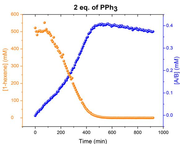
Fig. 10 Profiles of catalyst species from quantitative  $^{31}\text{P}\{^1\text{H}\}$  FlowNMR (upper) and 1-hexene concentration from quantitative  $^1\text{H}$  FlowNMR (lower) during the hydroformylation of 1-hexene under 10 bar of  $\text{CO}/\text{H}_2$  (1:1) at  $50^\circ\text{C}$  catalysed by  $[\text{Rh}(\text{acac})(\text{CO})_2] = 2.5$  mM and  $[\text{PPh}_3] = 5$  mM in 22.4 mL of non-deuterated toluene using the temperature gradients shown in Fig. 7.
