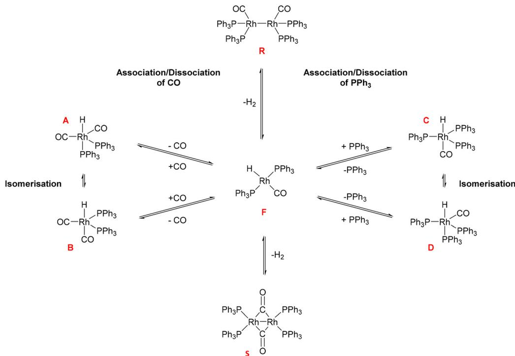
Scheme 2 Exchange equilibria between A/B and C/D in the presence of syngas and excess PPh<sub>3</sub> (dimers R and S will be discussed in more detail below; F has not been observed experimentally).
