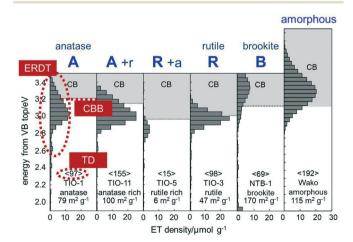
Fig. 1 Energy-resolved distribution of electron traps (ERDT)/ conduction-band bottom (CBB) patterns of representative commercial titania samples of anatase (A/a), rutile (R/r), brookite (B), amorphous and their mixtures. "A + r" and "R + a" show anatase-rich and rutile-rich, respectively, anatase-rutile mixtures.
