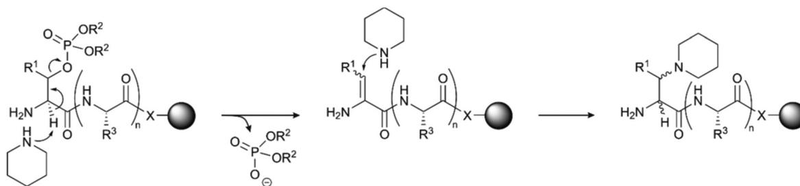
Fig. 3 Mechanism of piperidine mediated  $\beta$ -elimination of the double protected phosphate group from the side chains of serine ( $R^1 = H$ ) or threonine ( $R^1 = CH_3$ ) and formation of the piperidinium-adduct.  $R^2$  is the protecting group on the phosphate (see Table 1) and  $R^3$  represents the generic side chain of an amino acid. The nature of X depends on the functionalisation of the resin.
