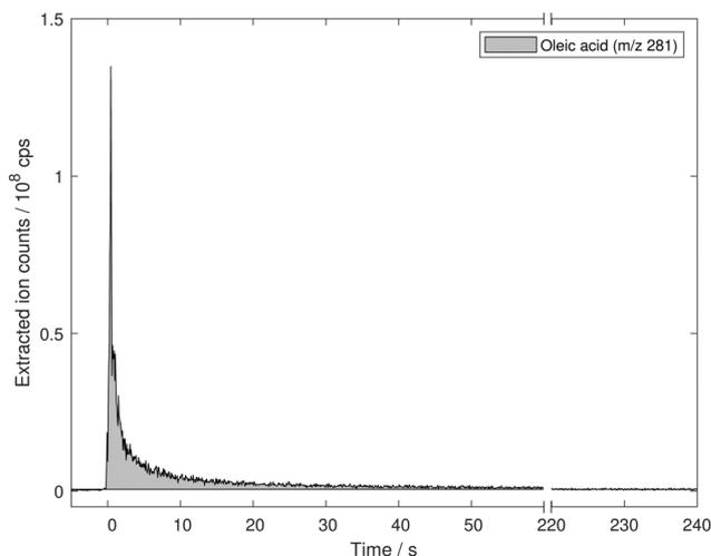
**Fig. 9** Extracted ion count for  $m/z$  281 from the evaporation of a single oleic acid droplet at 190 °C. After a sharp increase with the introduction of the droplet in the evaporation unit the signal intensity decays as the droplet shrinks and reaches background values before the end of the experiment at 240 s. The area below the curve corresponds to the amount of oleic acid in the drop.
