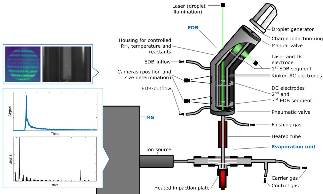
**Fig. 2** Schematic representation of the instrumentation. In the electrodynamic balance (EDB), charged particles are stored and aged under specific reaction conditions (ozone mixing ratio and reaction time). Subsequently, single particles are transferred to the evaporation unit and the resulting gas-phase compounds are transported to the ionisation region and analysed by mass spectrometry (MS). Parts are not drawn to scale.
