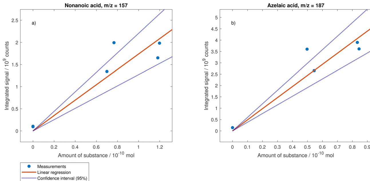
**Fig. 11** Calibration curves for nonanoic acid (a) and azelaic acid (b). Mixed droplets with different droplet compositions were used. For the calculation of the amount of substance, the molar volume was used and a refractive index of 1.46 was assumed for all droplets. The linear regression was forced through zero.
