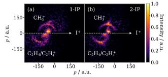
Fig. 5 Newton diagrams for the breakup of (a)  $1-IP^{2+/3+}$  and (b)  $2-IP^{2+/3+}$ into  $(I^+ + CH_3^+ + C_2H_4/C_2H_4^+)$ . The correlation of the  $I^+$  and  $CH_3^+$ momenta has been calculated using a contingent covariance analysis. The momentum of the third fragment, assumed to be  $C_2H_4$  or  $C_2H_4^+$ , is deduced through momentum conservation in this frame
