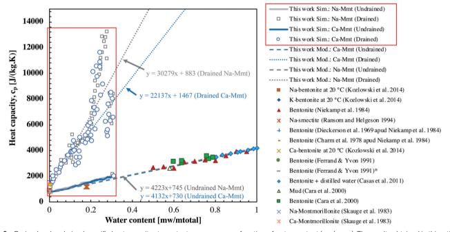
Fig. 9 Drained and undrained specific heat capacity at constant pressure  $c_p$  as a function of water content ( $m_w/m_{\text{total}}$ ). The results obtained in this article from molecular simulations concerning Na-Mmt and Ca-Mmt are shown inside the red boxes. These results are extrapolated to larger water content following the mixing rule (dashed lines, Ca-Mmt and Na-Mmt results are superposed). Drained  $c_p$  is computed considering the mixing of hydration states.
