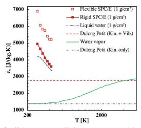
Fig. 4 Specific heat capacity  $c_v$  of bulk water: comparisons of simulations results using rigid and flexible SPC/E at a constant density as a function of the temperature with experimental data from the NIST database. Dulong-Petit estimates regarding only kinetics contribution  $C_v = (6/2) N_w k$ , and both kinetics and internal vibrations ( $C_v = 6N_w k$ ) are shown together with experimental measurements of water vapor as a function of the temperature.
