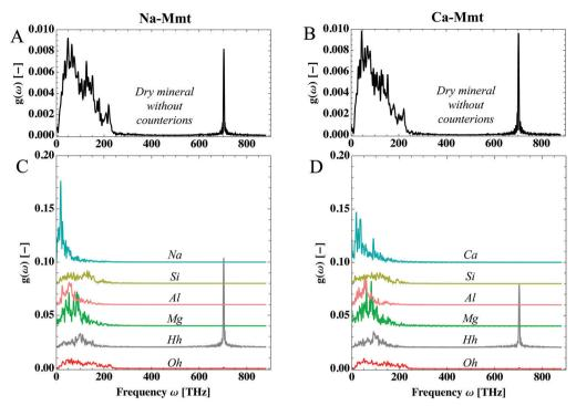
VDOS of dry mineral Na-Mmt (left) and Ca-Mmt (right): (A) and (B) total VDOS of the dry mineral; (C) and (D) VDOS per species.
