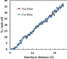
Fig. 3 Water content in terms of the number of water molecules  $N_{\rm w}$  per unit cell ( $[Si_{7.75}Al_{0.25}]_{tet}$  [Mg<sub>0.5</sub>Al<sub>3.5</sub>]<sub>oct</sub>O<sub>20</sub>(OH)<sub>4</sub>) as a function of the interlayer distance obtained from GCMC simulation of Na-Mmt and Ca-Mmt. The standard deviations of  $N_{\rm w}$  in the Ca-Mmt curve have the order of magnitude of the circles.
