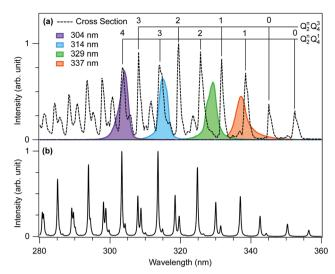
Fig. 1 (a) Experimental absorption cross section of  $D_2CO^{12}$  (black dotted line) and the UV spectra (solid lines) used in the present study. Strong absorption bands are assigned based on ref. 7, 12 and 13.  $Q_2$  and  $Q_4$  correspond to the C–O stretching mode and out-of-plane bending mode, respectively. (b) Simulated absorption spectrum.
