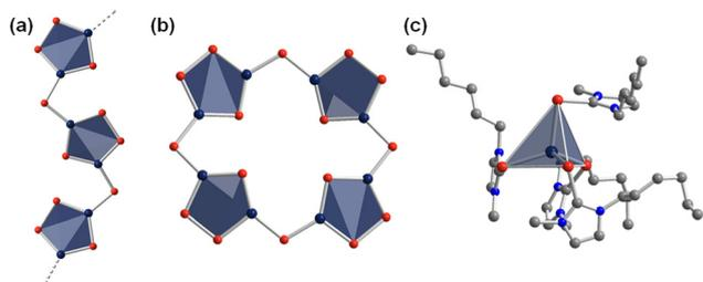
Fig. 3 Infinite zig-zag-strand structure of the anion  $1\text{D}-\{[\text{Hg}_2\text{Te}_4]^{2-}\}$  (a), molecular structure of the heavy metal porphyrinoid anion  $[\text{Hg}_8\text{Te}_{16}]^{8-}$  (b), molecular structure of the cationic complex  $[(\text{C}_6\text{C}_1\text{ImTe})_4\text{Hg}]^{2+}$  (c). Hydrogen atoms are omitted for clarity. Color code: Hg-dark blue, Te-red, C-grey, N-blue.
