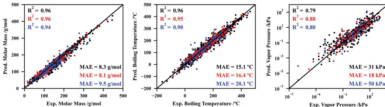
Fig. 2 Performance (predicted property vs. experimental property) of the convolutional neural networks developed in this work for molar mass (left), normal boiling temperature (middle), and vapor pressure at 25 °C (right). Black, red, and blue colors represent the results for the training, validation, and testing sets, respectively. The coefficient of determination ( $R^2$ ) and mean absolute error (MAE) are also included.
