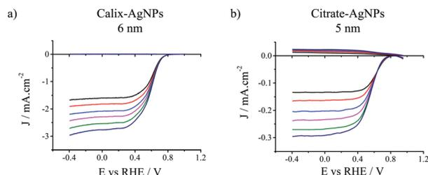
**Fig. 1** RRDE voltammetric curves in O<sub>2</sub>-saturated 0.1 M KOH solution of GC disk electrodes modified with either (a) 6 nm calix-AgNPs or (b) 5 nm citrate-AgNPs (bottom curves). Ring electrode (top curves): Pt. *v* = 10 mV s<sup>-1</sup>. *ω* = 400, 600, 900, 1200, 1600, 2000 rpm. *E*<sub>ring</sub> = 1.70 V *vs.* RHE. Normalized current density per electrochemically active surface area are reported.
