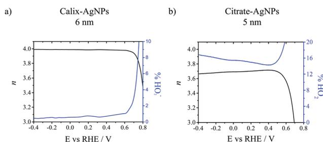
**Fig. 2** Potential dependence of the number of electrons *n* (black lines) and the yield of HO<sub>2</sub><sup>-</sup> (blue lines) produced during ORR experiments for (a) 6 nm calix-AgNPs and (b) 5 nm citrate-AgNPs.
