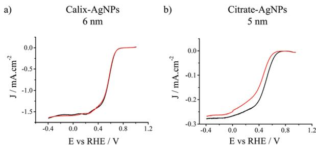
**Fig. 3** Linear sweep voltammetry (LSV) curves recorded at 1600 rpm on (a) 6 nm calix-AgNPs and (b) 5 nm citrate-AgNPs before (black curves) and after (red curves) stability test in  $O_2$ -saturated 0.1 M KOH solution. Normalized current density per electrochemically active surface area are reported.
