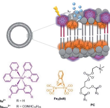
Fig. 28 A self-assembled bilayer preorganizes a Ru-photosensitizer and [FeFe]-hydrogenase mimic for light driven proton reduction. Used with permission from ref. 119.
