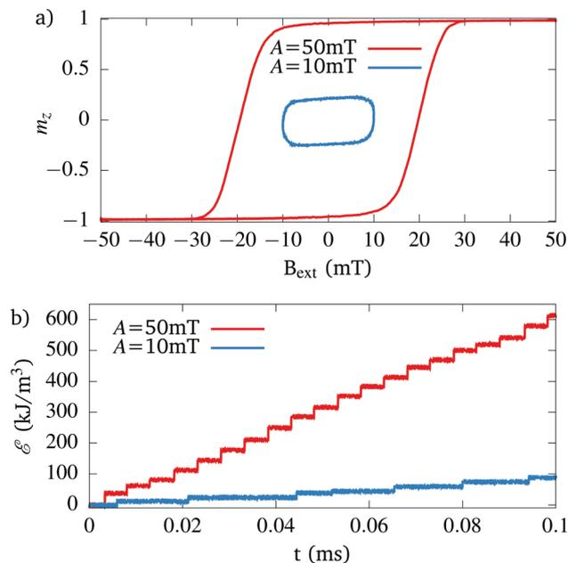
**Fig. 5** (a) Hysteresis loops for an ensemble of 10 000 particles, excited with a sinusoidal externally applied magnetic field with amplitudes of 10 mT (blue lines) and 50 mT (red lines). (b) Dissipated heat by a single particle as function of time for 10 periods of the field excitation.
