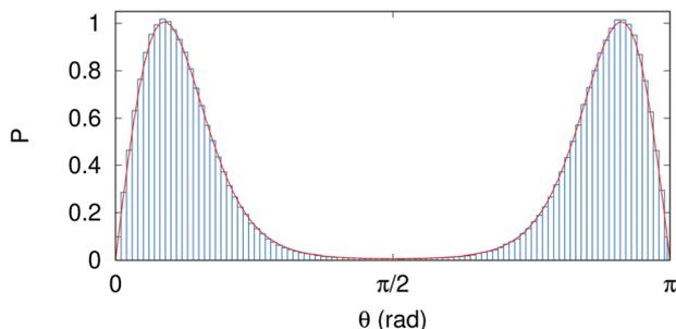
Fig. 2 Probability with maximum normalised to 1,  $P$ , to find the magnetisation under an angle  $\theta$  with respect to the anisotropy easy axis, as extracted from simulations (blue bars) and eqn (8) (red line).
