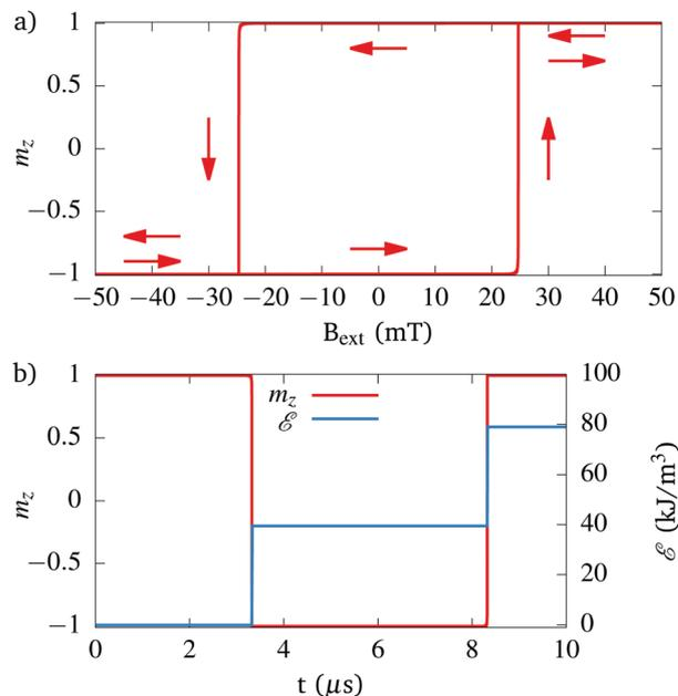
Fig. 4 (a) Hysteresis loop for a single domain particle in an externally applied field parallel with its anisotropy easy axis. (b) The magnetisation along the easy axis  $m_z$  and dissipated energy density  $\mathcal{E}$  as function of time for a single hysteresis loop. Heat only gets dissipated during the two switching events.
