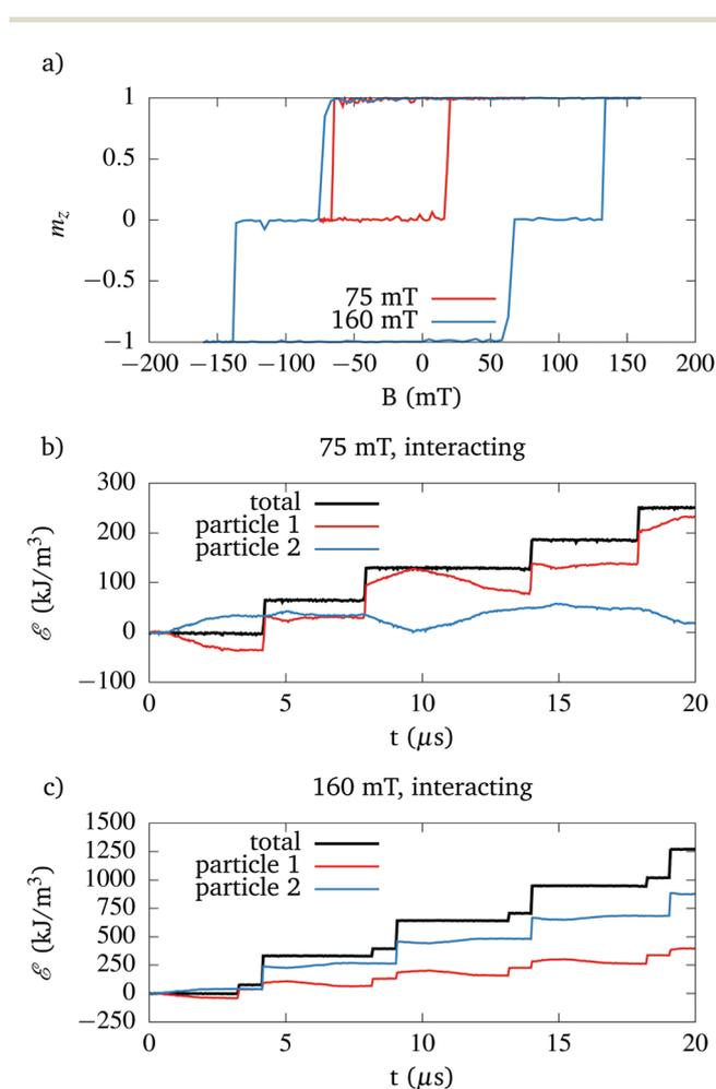
**Fig. 8** (a) Hysteresis loops for particles, excited with an sinusoidal externally applied magnetic field with amplitudes of 75 mT (red lines) and 160 mT (blue lines). (b) and (c) Dissipated heat by individual particles as function of time for 10 periods of the field excitation with amplitude 75 mT [panel (b)] and 160 mT [panel (c)], respectively. These figures correspond to the cases highlighted with filled dots in Fig. 6.
