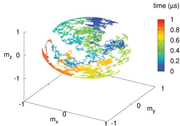
**Fig. 1** Magnetisation direction, depicted on the unit sphere, as function of time (colour coded) for an isotropic magnetic nanoparticle at nonzero temperature. The magnetisation performs a random walk without preferential direction.
