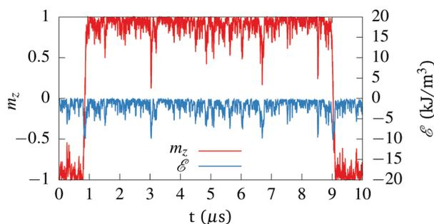
Fig. 3 Magnetisation along the anisotropy easy axis (left  $y$ -axis, red line) and energy density,  $\mathcal{E}$ , showing the heat extracted from and dissipated into the particle environment, as function of time. Note the two switching events around  $t = 1 \mu\text{s}$  and  $t = 9 \mu\text{s}$ .
