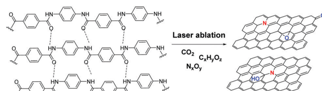
Fig. 2 Laser-induced transformation of Kevlar into graphene-functionalized material.
