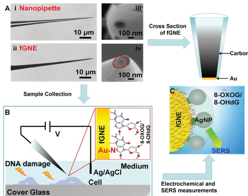
**Fig. 1** Schematic diagram of the experimental setup. (A) Optical (left) and SEM images (right) of the nanopipette (i and iii) and fGNE (ii and iv). The orifice pointed by the red circle indicates the successful deposition of gold on the carbon nanoelectrode. (B) Diagram of the fGNE collecting DNA damage products (only the 8-OHdG structure is shown here) from individual cells. (C) Illustration of SERS detection of cellular DNA damage products on the fGNE with AgNPs.
