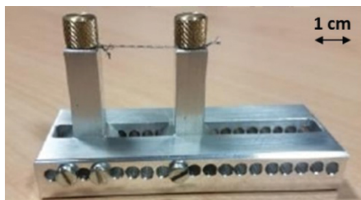
Fig. 2 Picture of the lab-made device to stretch yarn for SEM observation.
