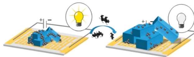
Fig. 5 Switchable MIL-53-carbon additive composite for CO 2 sensing. 25
