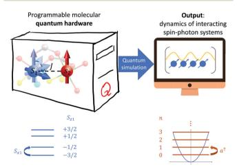
Fig. 1 Scheme of the molecular quantum simulator. Left: hardware setup, consisting of a qudit spin  $\mathcal{S}_1$  coupled by exchange interaction  $\mathcal{J}$  to a spin  $s_2 = 1/2$ . Right: target spin-photon model. In the bottom part of the figure we qualitatively also sketch the mapping between the qudit, with all the transitions made energetically distinguishable by the combined effect of Zeeman and zero-field splitting interactions, and the boson field.
