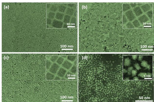
**Fig. 2** (a) TEM images of the QDs: (a) green light emitting pristine  $\text{CsPbBr}_3$  QDs, (b) blue light emitting  $\text{CsPb}(\text{Br}_{1-x}\text{Cl}_x)_3$  QDs, (c) blended cyan light emitting  $\text{CsPb}(\text{Br}_{1-x}\text{Cl}_x)_3$  QDs, and (d) red light emitting CIS QDs.
