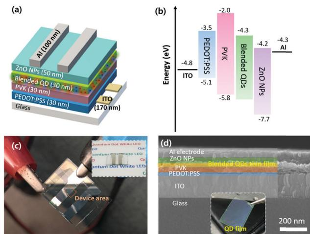
**Fig. 1** (a) Schematic structure of the QD-based WLED device. (b) Energy band structure of the QD-based WLED device. (c) Photo image of WLEDs. The inset shows the spin-coated QD thin films on a PVK/PEDOT:PSS/ITO/glass substrate. (d) Cross-sectional high-resolution SEM image of the full structure of the QD-based WLED device. The inset shows the spin-coated QD thin films exhibiting uniform and flat surfaces.
