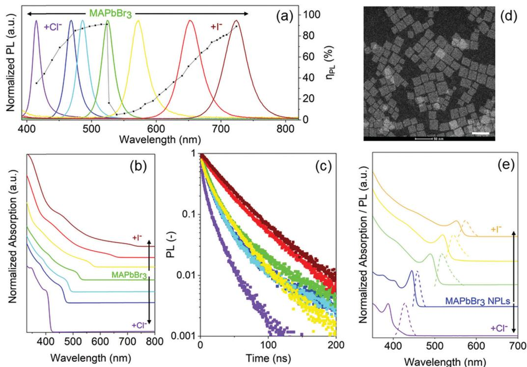
Fig. 3 Normalized (a) PL and (b) absorption spectra of the parent MAPbBr<sub>3</sub> and mixed-halide perovskite NCs together with their  $\eta_{\text{PL}}$ . (c) Time-resolved photoluminescence (TRPL) responses of the synthesized NCs. (d) Representative transmission electron micrograph of 2D MAPbBr<sub>3</sub> NPLs (scale bar: 50 nm). (e) Absorption (solid lines) and PL (dashed lines) of the LASPS synthesized mixed-halide perovskite NPLs.
