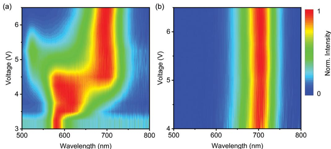
Fig. 5 EL spectra of KI-exchanged MAPb(Br/I)<sub>3</sub> under electrical stress. (a) The evolution of EL spectra as a function of driving voltage. (b) EL spectra of the color-stable mixed-halide MAPb(Br/I)<sub>3</sub> NCs after applying a reverse bias of  $-4$  V for 20 minutes.
