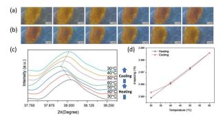
Fig. 8 (a and b) Temperature-induced color change of the CC crystal with heating and cooling cycles. Temperature-dependent XRD of CC: (c) Expansion of  $2\theta = 38.1^{\circ}$  reflection at different temperatures. (d) d-spacing calculated from the  $2\theta$  values extracted from the XRD patterns at different
