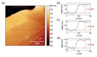
Fig. 3 (a) AFM topography image of the C3 perovskite bulk single crystal on the (002) plane (scale bars: 1 µm). (b-d) Height profiles of three regions A-C, respectively, of C3 perovskite bulk single crystal along the (002) facet
