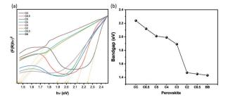
**Fig. 5** Band gap determination of Cu-perovskites (a) Kubelka–Munk function plot. (b) Band gap energy values of Cu-perovskite crystals extracted from the Kubelka–Munk function.
