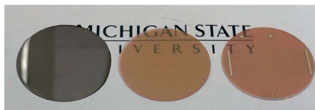
Fig. 2 A completely Pt-covered PCO|YSZ sample (left), an uncovered PCO|YSZ sample (middle), and a partially Pt-covered PCO|YSZ sample (right). Note, each sample was 25.4 mm in diameter.
