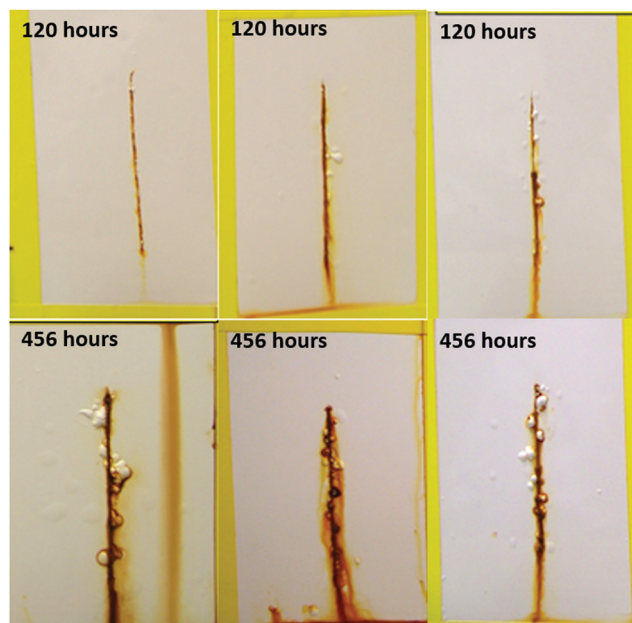
Fig. 10 Blisters develop about a scribe introduced to three different coating formulations undergoing salt spray test. This progression is in agreement with the qualitative description of a surface undergoing saponification about the scribe, followed by blistering driven by osmotic pressure generated by corrosion products. However, for this to happen, defects must become sealed by corrosion products.
