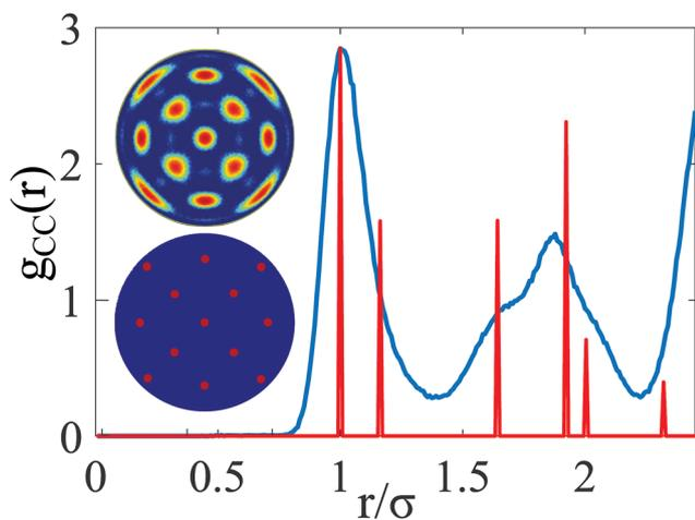
Fig. 3 Cluster-cluster pair distribution function ( $g_{cc}(r)$ ) and bond-orientational order diagram (BOOD) measured using the center of mass of the clusters in the cluster-crystal obtained at  $\rho^* = 0.05$  and  $T^* = 0.2$ . These CC-PDF and BOOD are compatible with those of the BCC crystal lattice (also shown for comparison).
