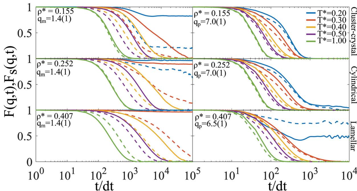
Fig. 10 Coherent ( $F(q,t)$ , solid lines) and incoherent ( $F_s(q,t)$ , dashed lines) intermediate scattering functions evaluated at the microphase ( $q_m$ ) and at the particle ( $q_p$ ) scales at different temperatures along three isochores:  $\rho^* = 0.155$  (cluster-crystal),  $\rho^* = 0.252$  (cylindrical phase) and  $\rho^* = 0.407$  (lamellar phase).
