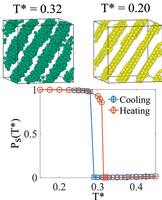
Fig. 6 Top row: Representative configurations of liquid ( $T^* = 0.32$ , left) and crystalline ( $T^* = 0.20$ , right) lamellar phases at  $p^* = 0.50$ . Particles with solid local environments are colored in yellow and particles with liquid local environments in green. Bottom panel: average fraction of solid particles ( $P_s$ ) as obtained using the Lechner and Dellago local order parameter.<sup>28</sup>
