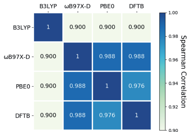
Fig. 6 Spearman correlation between DFTB and DFT predictions of specific storage energy for norbornadienes with different exchange-correlation functionals.
