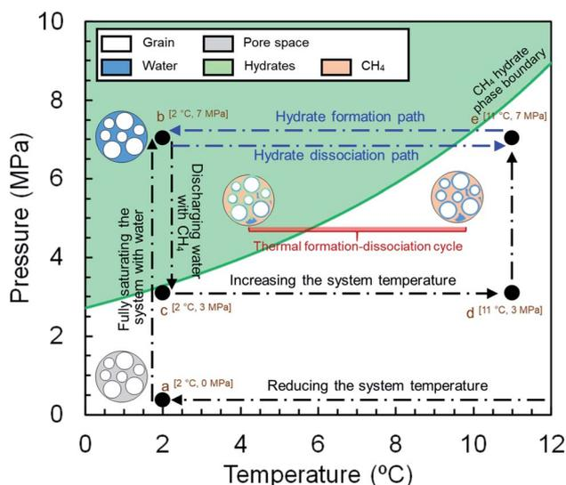
Fig. 2 Schematic diagram of the experimental procedure.
