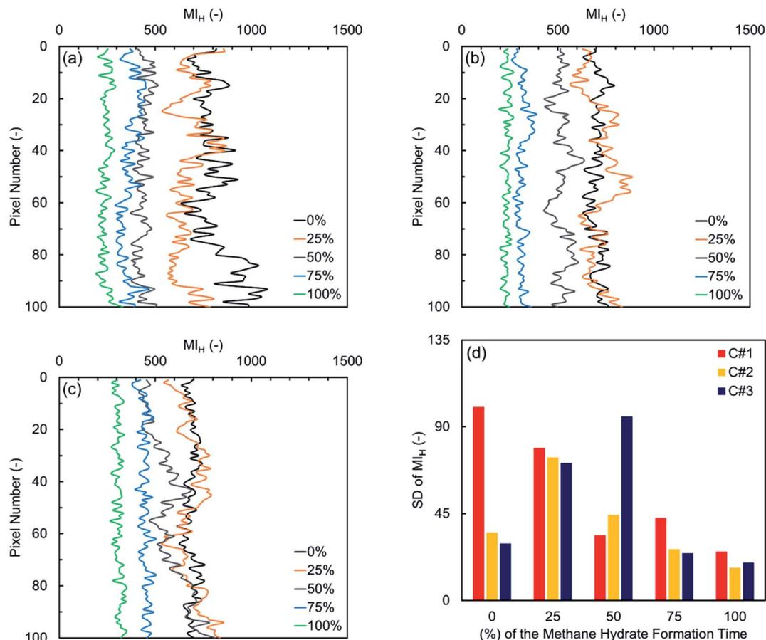
Fig. 7  $MI_H$  values versus the pixel number in the vertical direction initially and at the end of four quarters of the hydrate formation time of the (a) first, (b) second, and (c) third thermal cycles for the natural sediment sample, together with (d) their standard deviation (SD).
