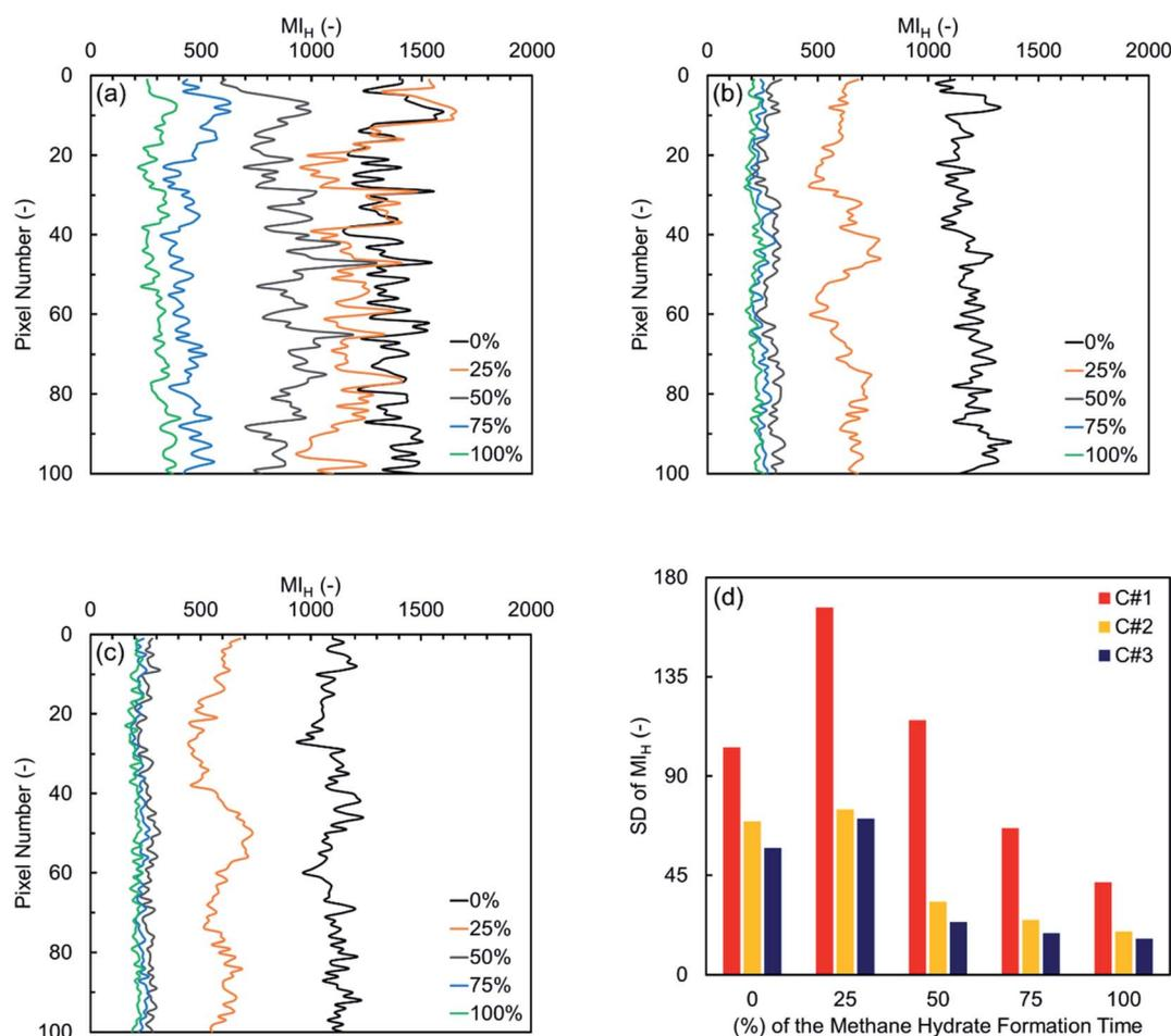
Fig. 6  $MI_H$  values *versus* the pixel number in the vertical direction initially and at the end of four quarters of the hydrate formation time of the (a) first, (b) second, and (c) third thermal cycles for the synthetic sediment sample, together with (d) their standard deviation (SD).
