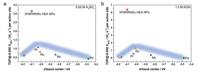
Fig. 6 TOF value at  $-0.05 \, V_{RHE}$  as a function of the experimental d-band center of the tested catalysts in (a)  $0.05 \, M \, H_2SO_4$  and (b)  $1.0 \, M \, KOH$  solutions. The d-band center is relative to the Fermi level. The light blue regions show the trend of the activity following d-band center theory.
